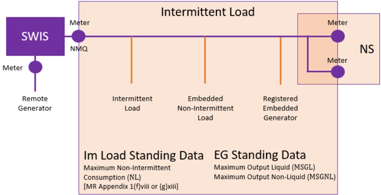
The purpose of this section is to define the Metered Schedule Quantities for each of the components. To do this, various standing data relating to the Intermittent Load and the embedded generator is used; however, the first step is to perform the following preliminary calculations to derive  $AMQ_{FI}$ .
