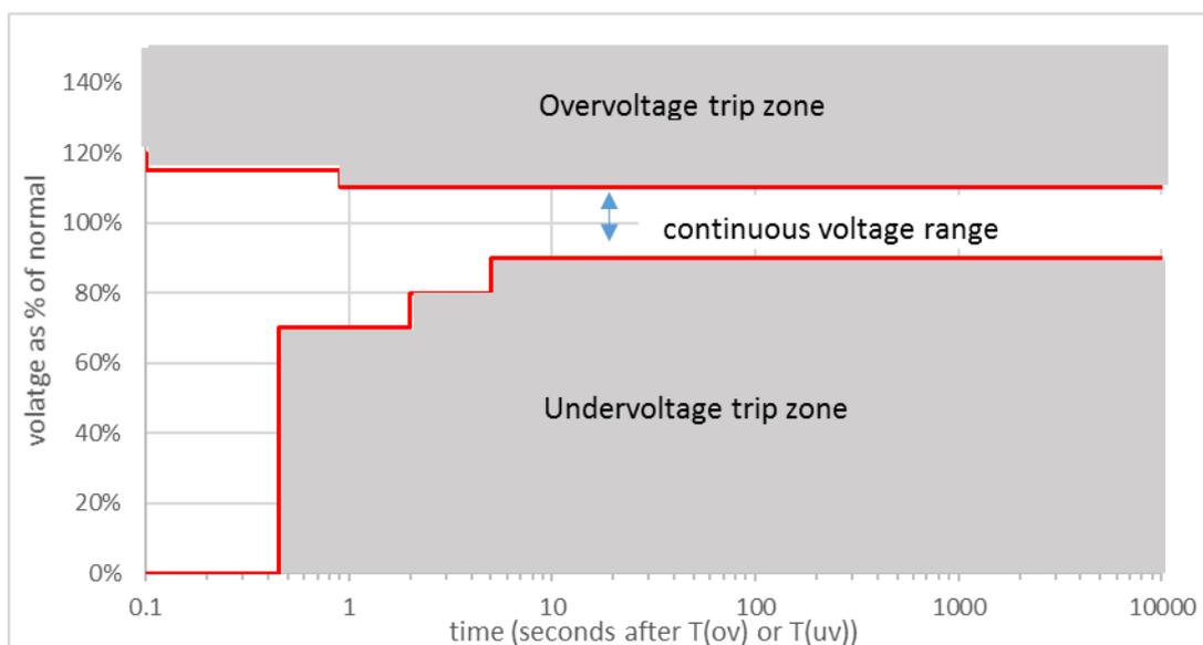
Figure 11 : *Voltage* variations that a *generating system* must ride through to meet the minimum standard
