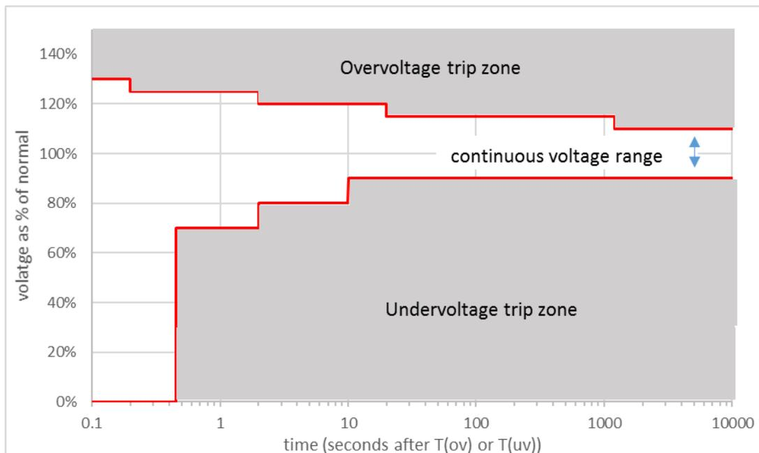
**Figure 10 : Voltage variations that a *generating system* must ride through to meet the ideal standard**
