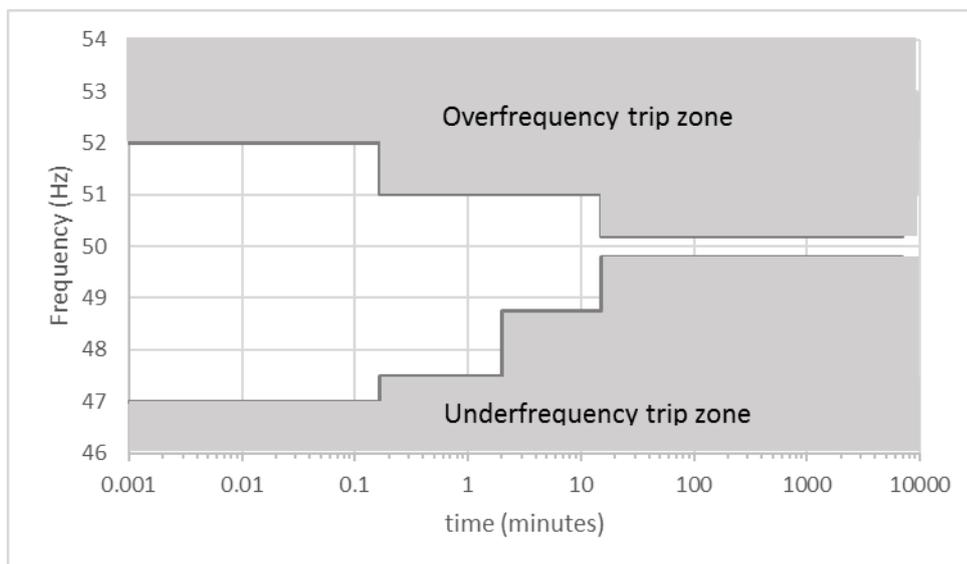
**Figure 8 : Frequency variations that a *generating system* must ride through to meet the minimum standard**
