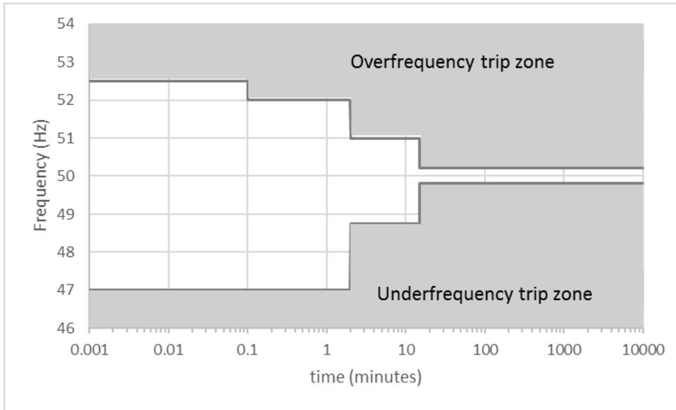
**Figure 6 : Frequency variations that a *generating system* must ride through to meet the ideal standard**
