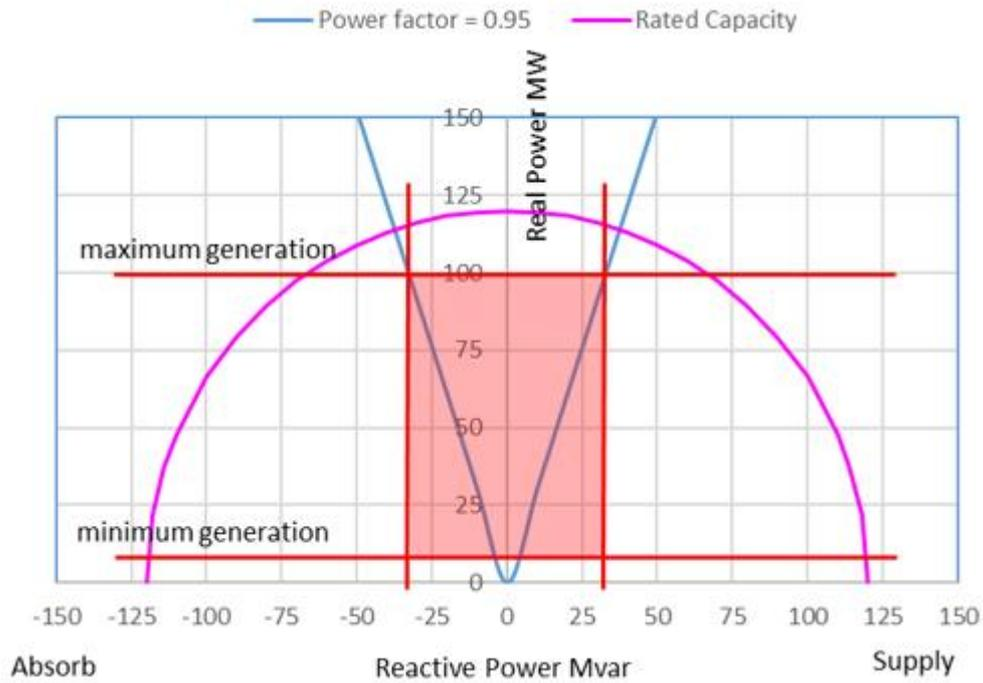
Figure 4 : *Reactive power* capability required to meet the minimum standard
