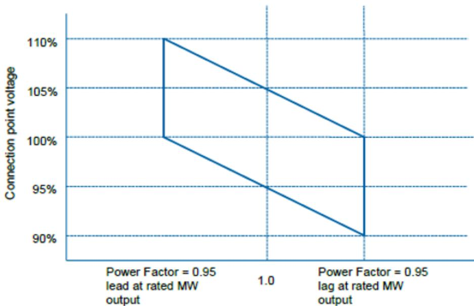
Figure 5 : Relaxation of *reactive power* requirement with *connection point voltage*
