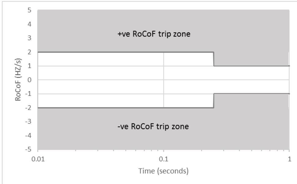
**Figure 9 : RoCoF that a *generating system* must ride through to meet the minimum standard**
