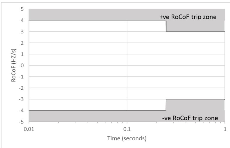
**Figure 7 : RoCoF that a *generating system* must ride through to meet the ideal standard**
