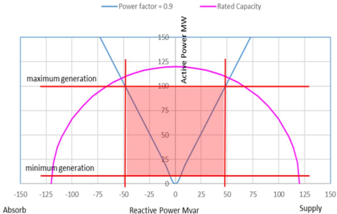
**Figure 2 : Reactive power capability required to meet the ideal standard**
