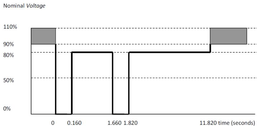
**Figure 12 : Connection point voltage during auto reclose operation**
