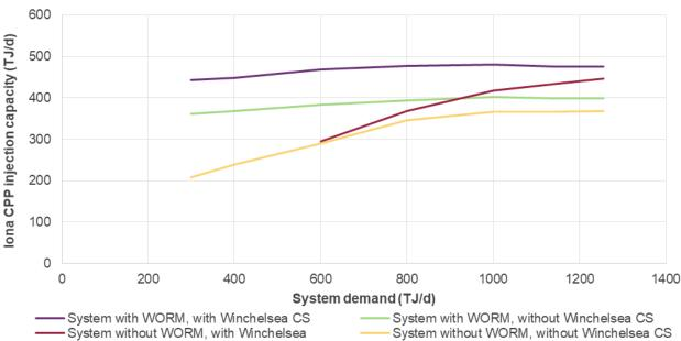
Figure 37 SWP injection capacity (including WTS demand) to Melbourne with the WORM (TJ/d)
