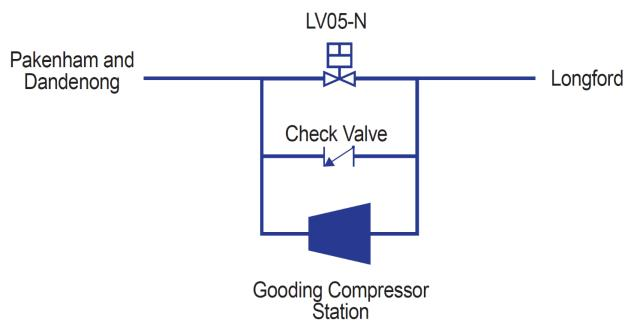
Figure 30 Gooding compressor station valve arrangement
