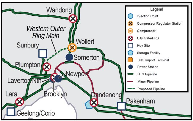
Figure 29 The Western Outer Ring Main system augmentation
