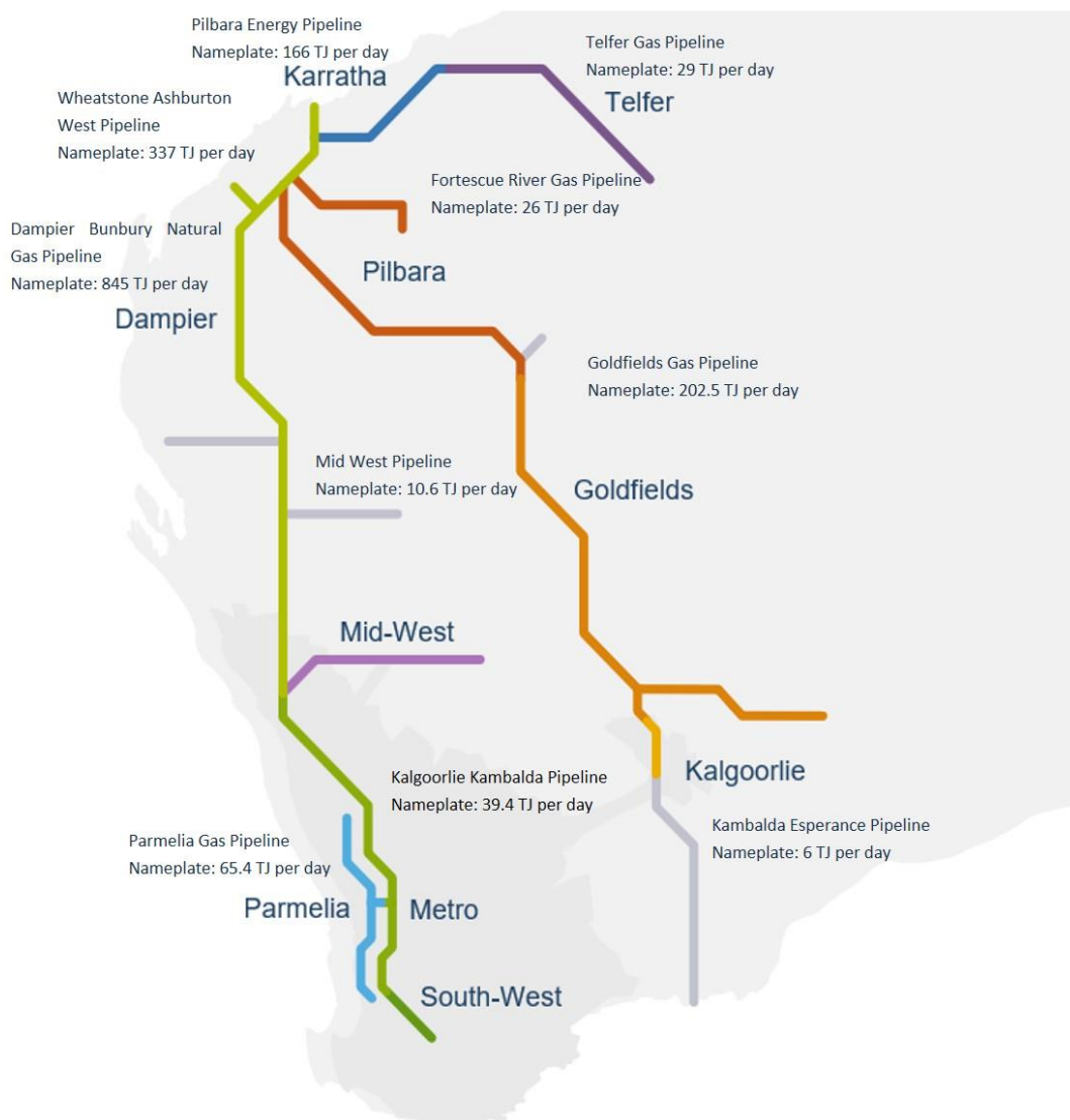
Figure 30 Gas transmission pipelines in WA
