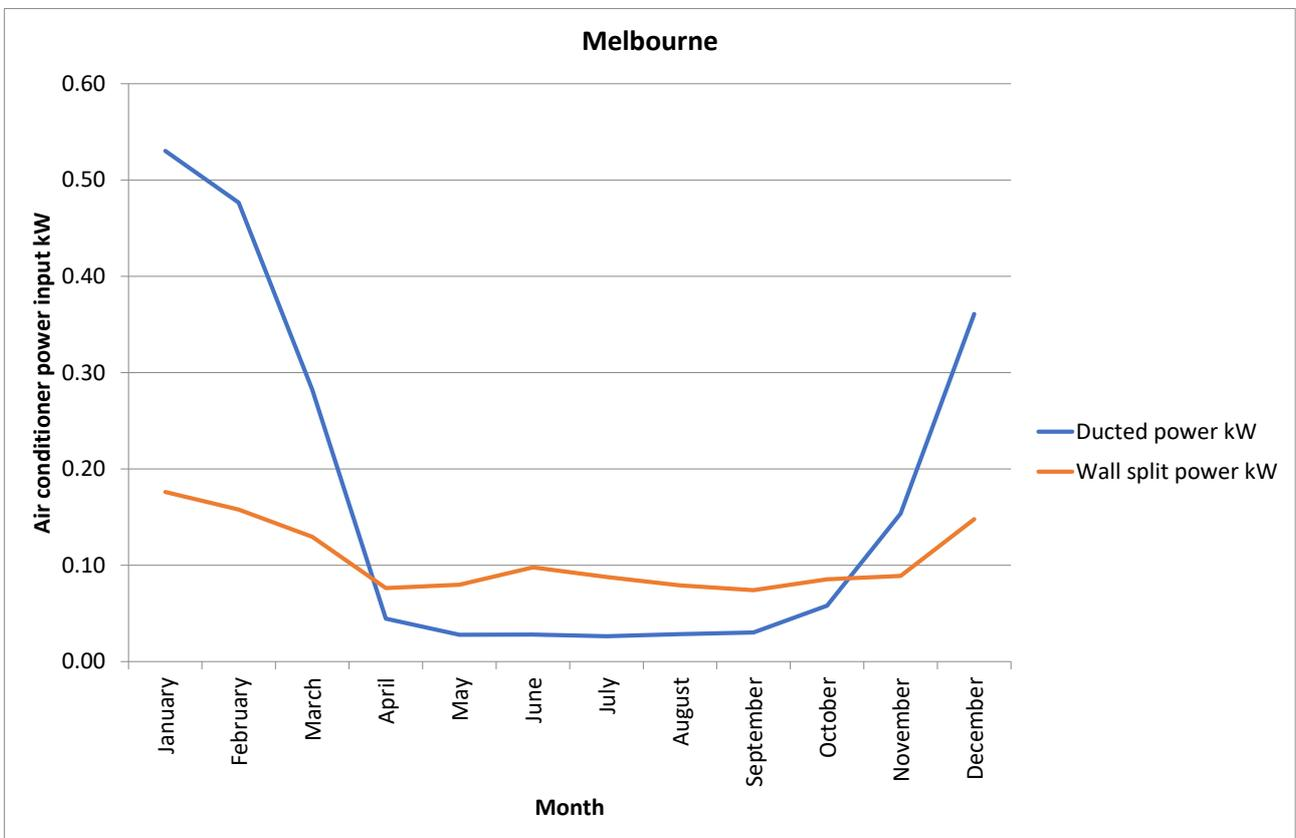
Figure 36: Seasonal power profile for ducted and split systems, Melbourne
