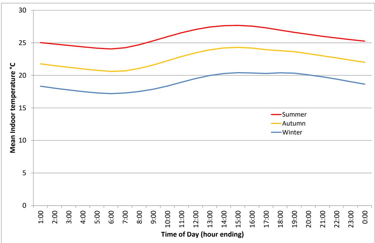
Figure 76: Seasonal indoor temperature profiles for houses in Brisbane (Harrington 2018)
