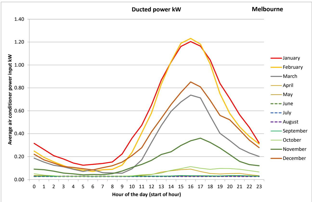
Figure 41: Time-of-day usage for ducted air conditioners by month, Melbourne
