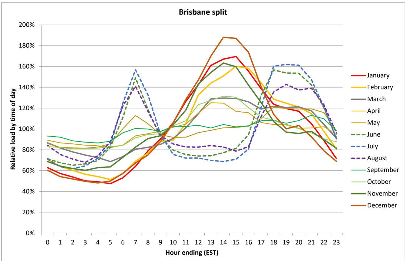
Figure 56: Relative time-of-day profile for split air conditioners, Brisbane
