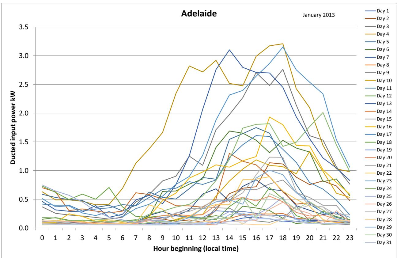
Figure 51: Daily power input traces for ducted air conditioners in Adelaide, January 2013
