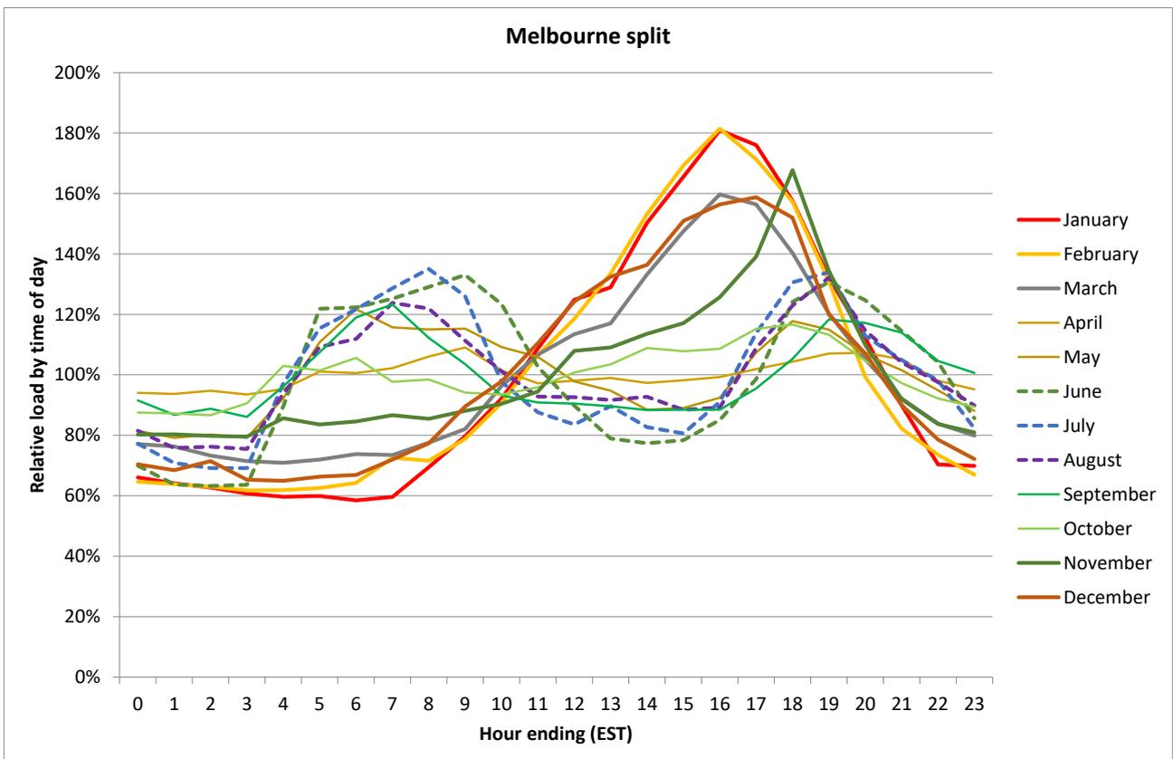
Figure 60: Relative time-of-day profile for split air conditioners, Melbourne
