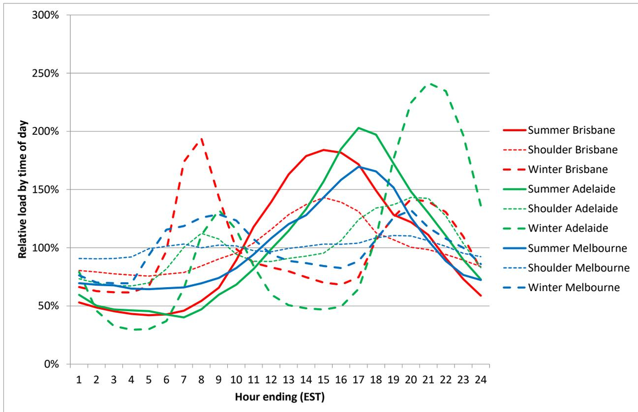
**Figure 61: Generic air conditioner time-of-day load shapes – residential main air conditioners**
