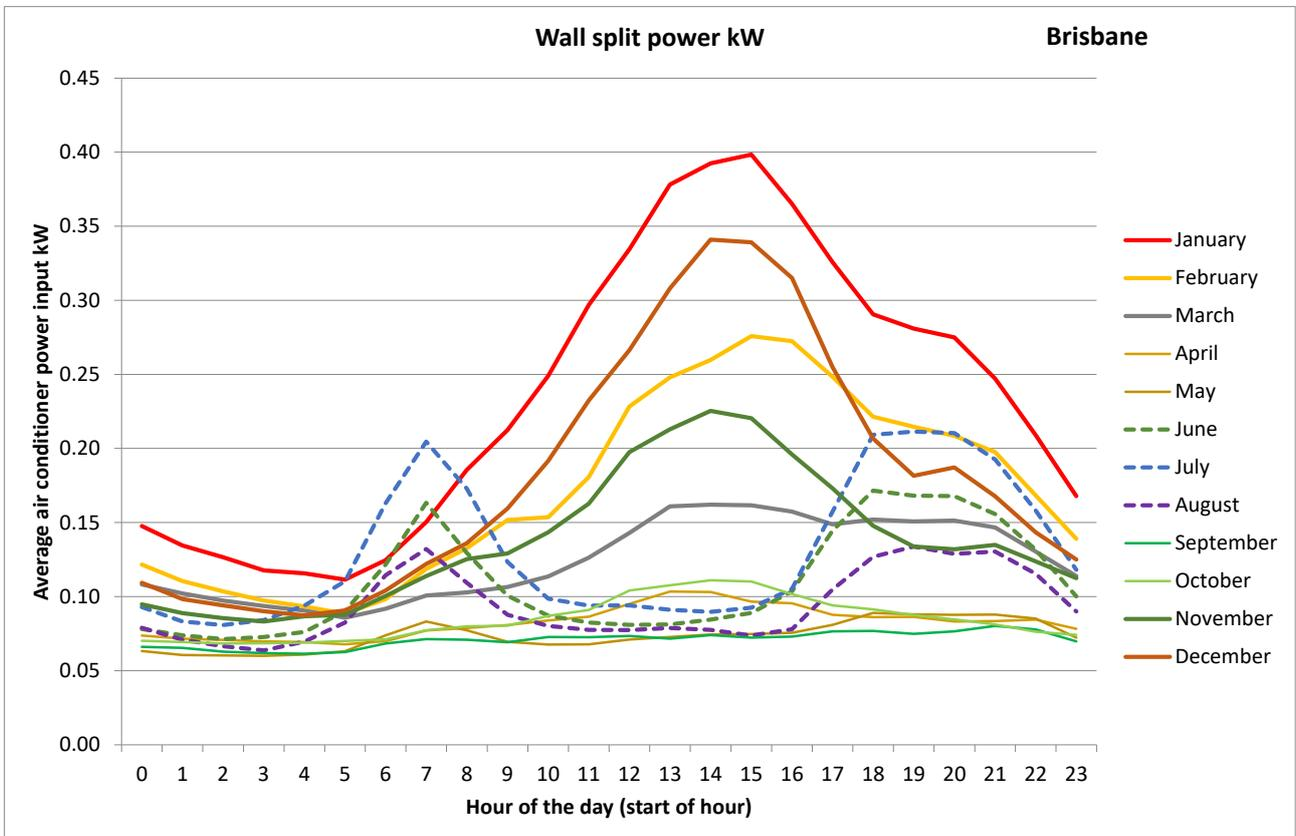
Figure 38: Time-of-day usage for split system air conditioners by month, Brisbane
