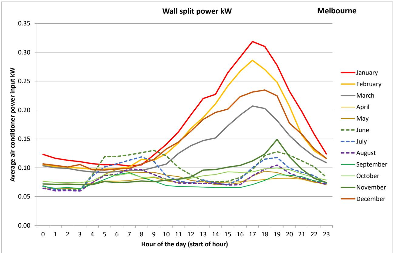
Figure 42: Time-of-day usage for split system air conditioners by month, Melbourne
