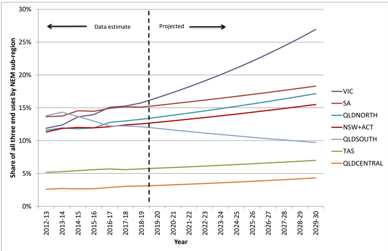
Figure 105: Projected share of energy for all air conditioners, household and commercial refrigeration based on trend data
