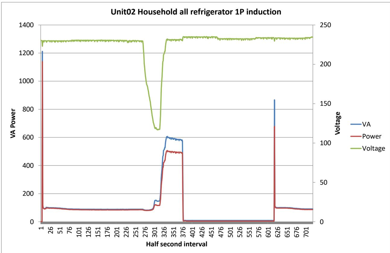
**Figure 20: Example of low voltage stall data for a household refrigerator**
