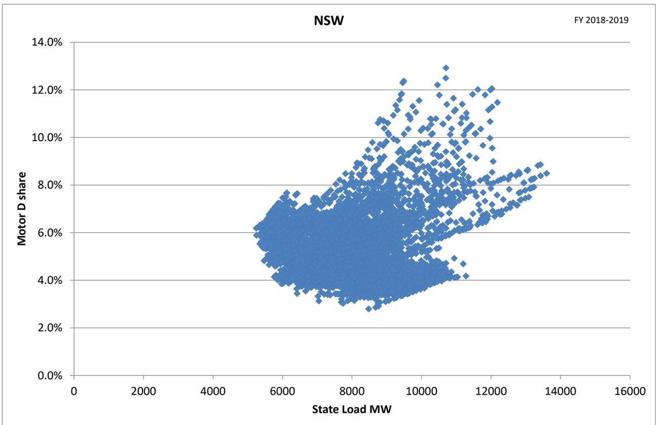
**Figure 103: Motor D share versus underlying system load for NSW and ACT in 2018-2019**
