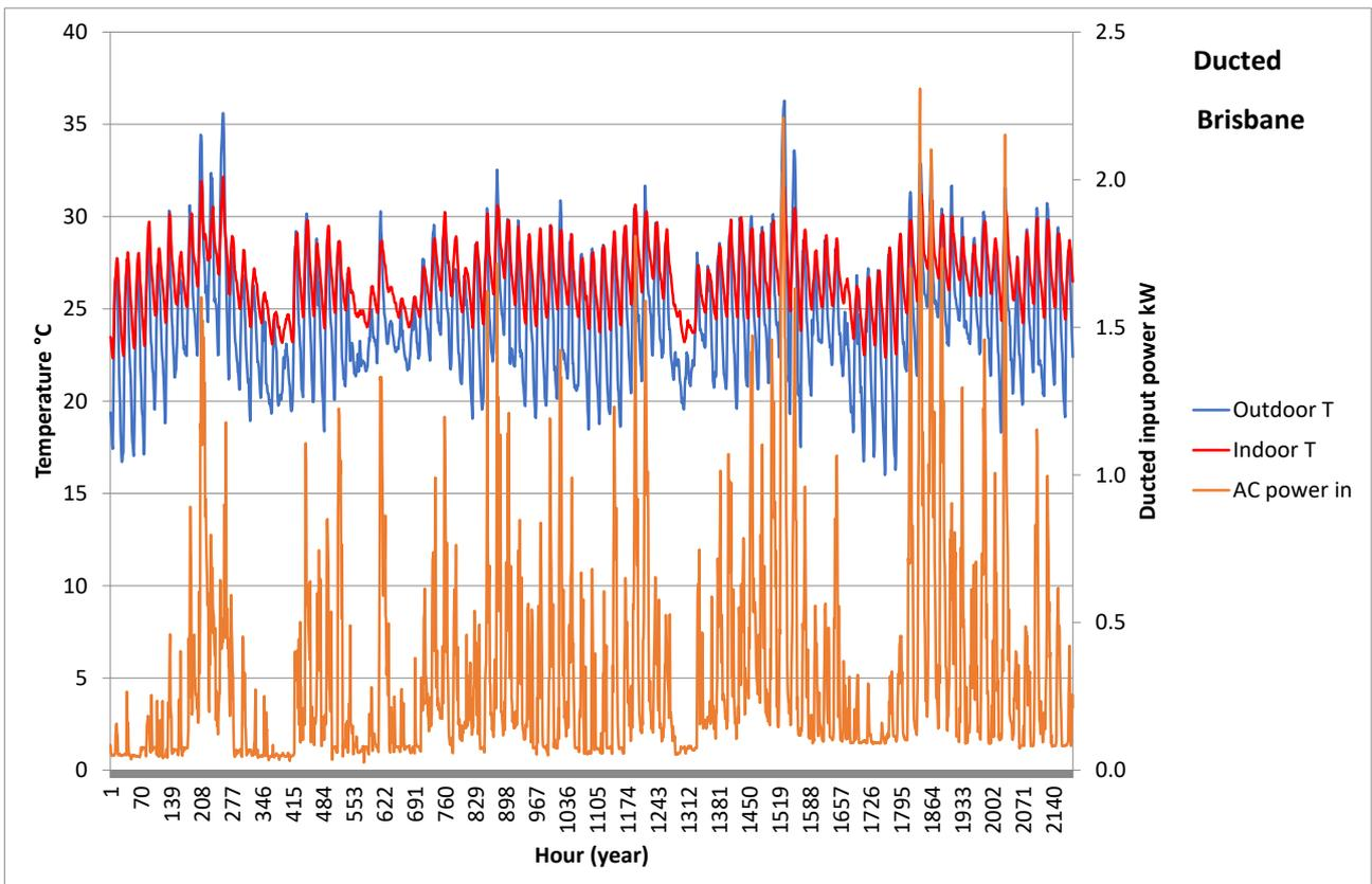
**Figure 44: Hourly temperature and ducted power data for Brisbane: Jan, Feb and Dec 2012**
