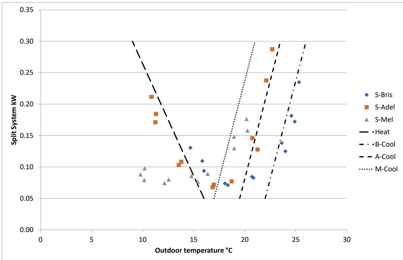
**Figure 54: Average monthly ducted air conditioner by outdoor temperature**
