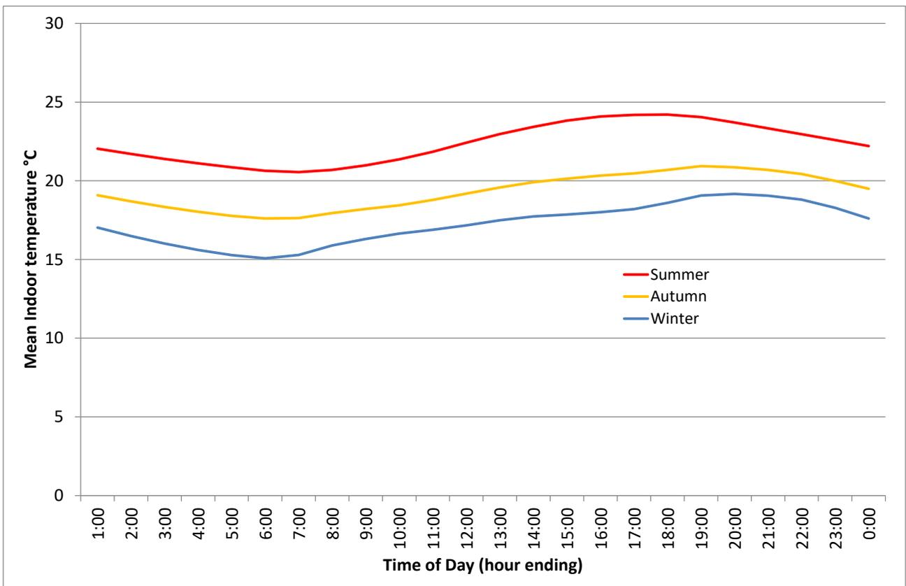
Figure 78: Seasonal indoor temperature profiles for houses in Melbourne (Harrington 2018)
