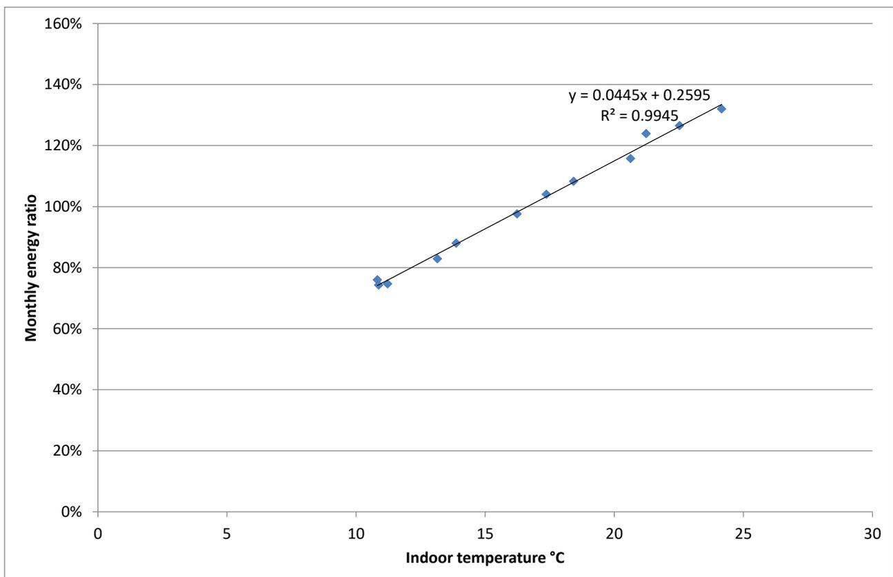
**Figure 87: Typical energy response to temperature changes for commercial refrigeration**
