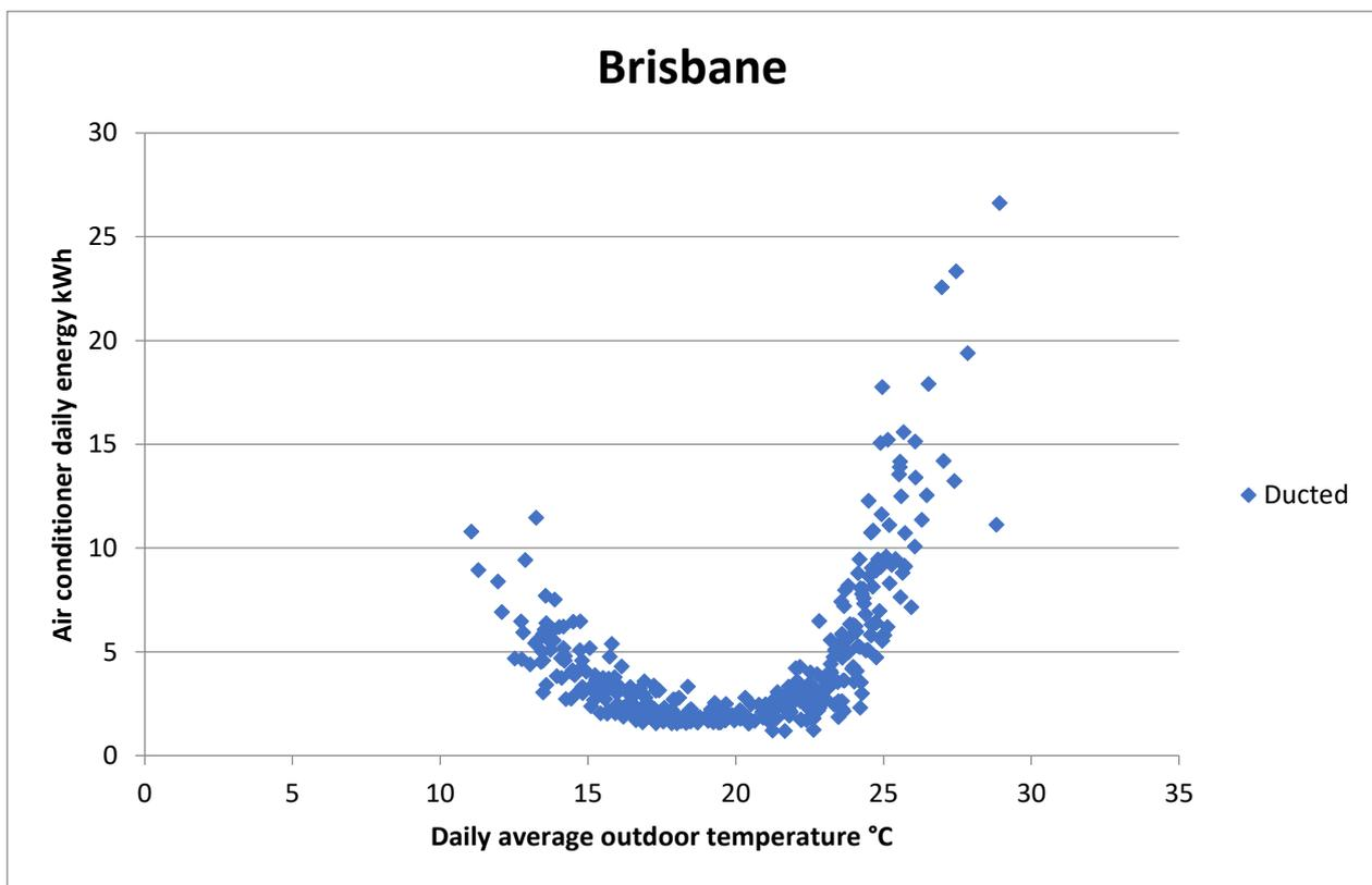
**Figure 50: Daily average outdoor temperature versus ducted air conditioner energy: Brisbane, 2012**
