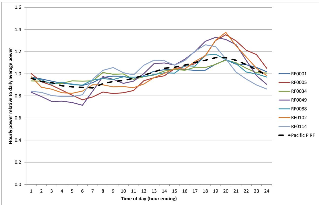
**Figure 80: Normalised time-of-day for a selection of refrigerators**
