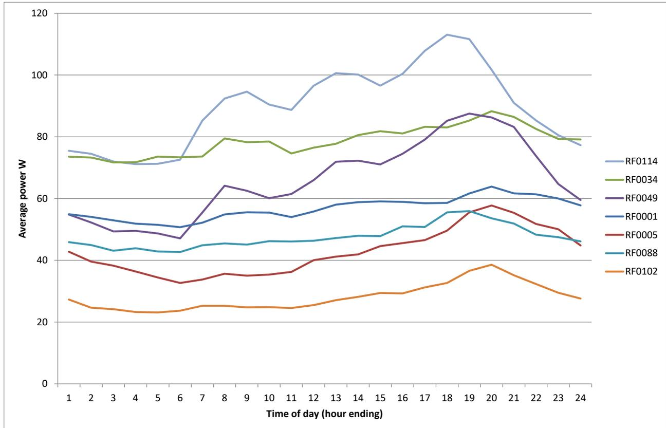
**Figure 79: Time-of-day average power for seven refrigerators (Harrington 2018)**
