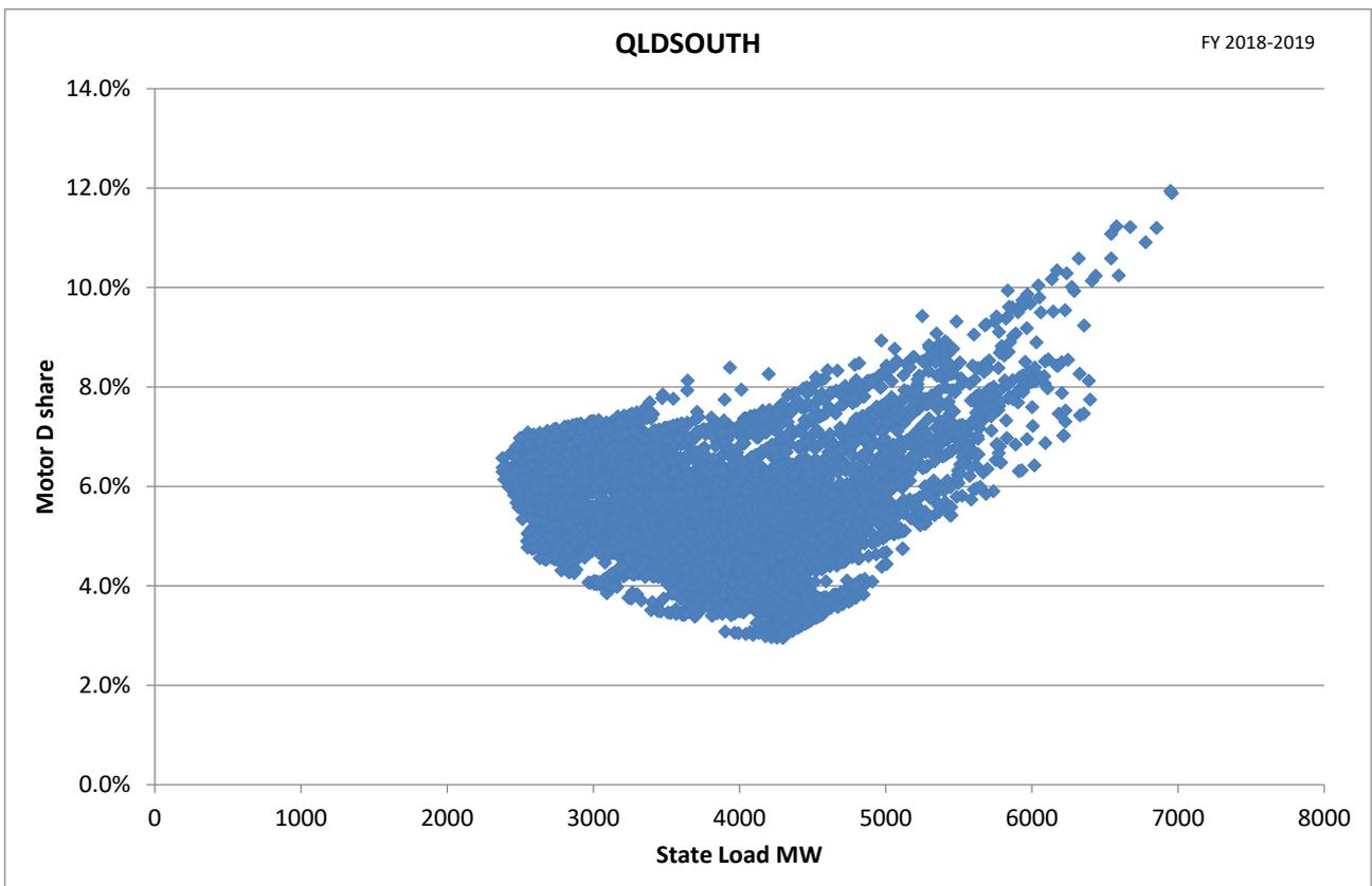
**Figure 104: Motor D share versus underlying system load for Queensland South in 2018-2019**
