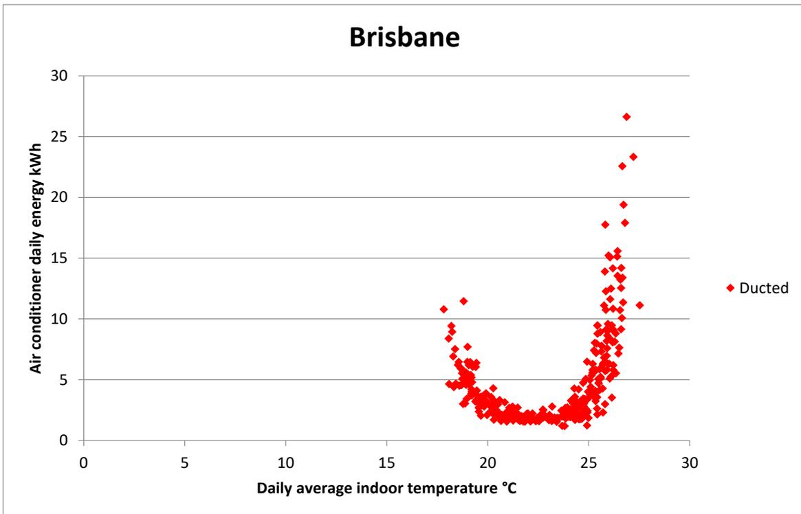
**Figure 49: Daily average indoor temperature versus ducted air conditioner energy: Brisbane, 2012**
