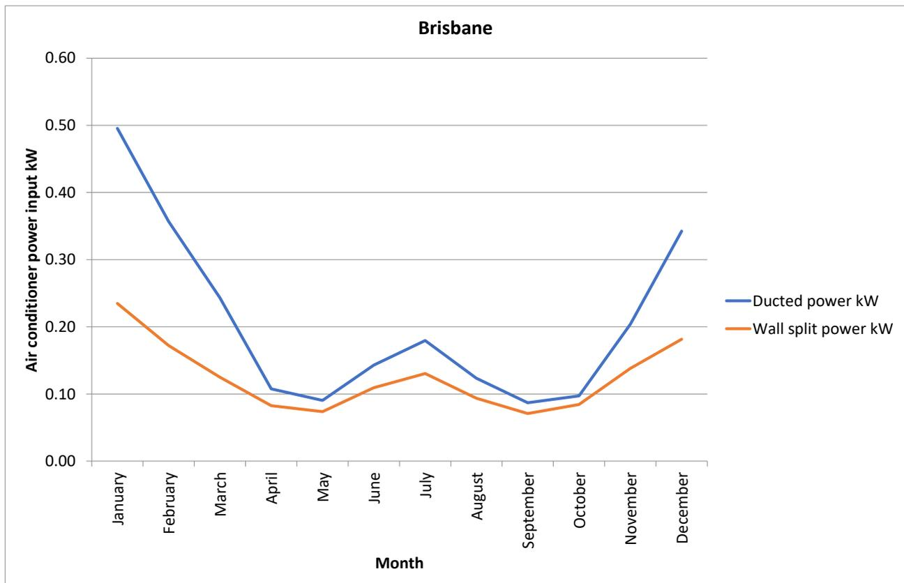
Figure 34: Seasonal power profile for ducted and split systems, Brisbane
