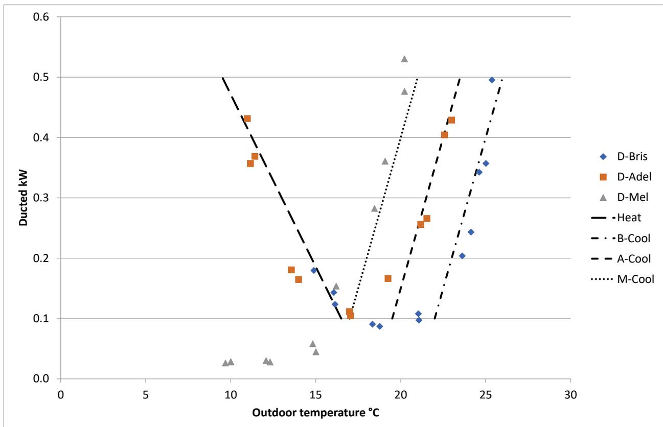
Figure 53: Average monthly ducted air conditioner by outdoor temperature
