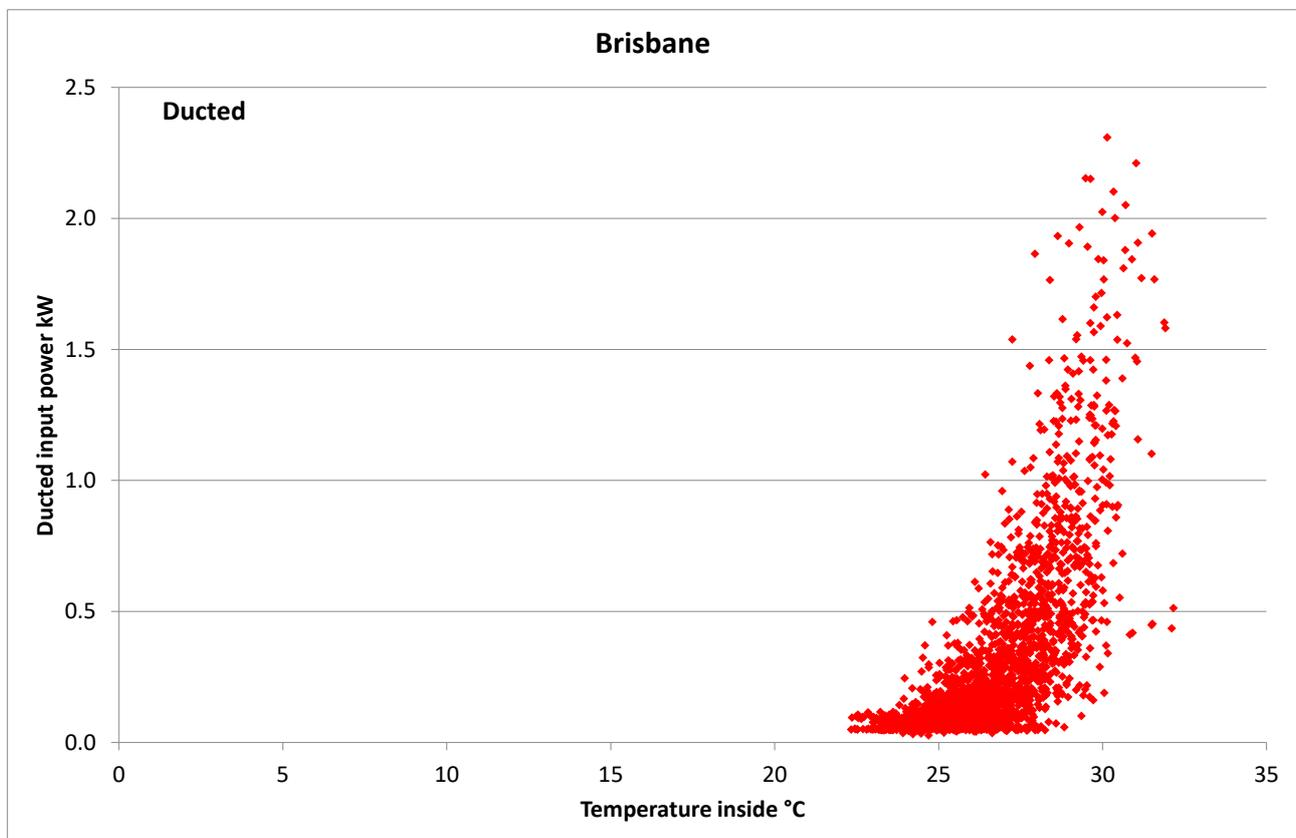
**Figure 47: Hourly indoor temperature vs ducted power data for Brisbane: Jan, Feb and Dec 2012**
