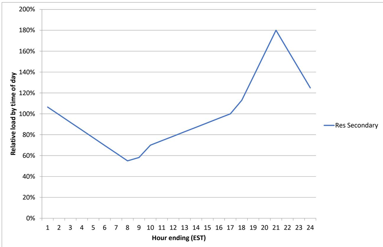
**Figure 62: Generic air conditioner time-of-day load shapes – residential secondary air conditioners**
