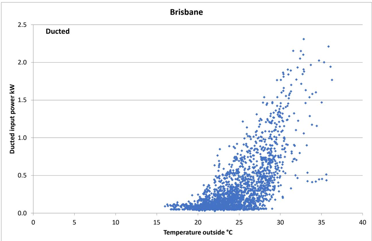
**Figure 48: Hourly outdoor temperature vs ducted power data for Brisbane: Jan, Feb and Dec 2012**
