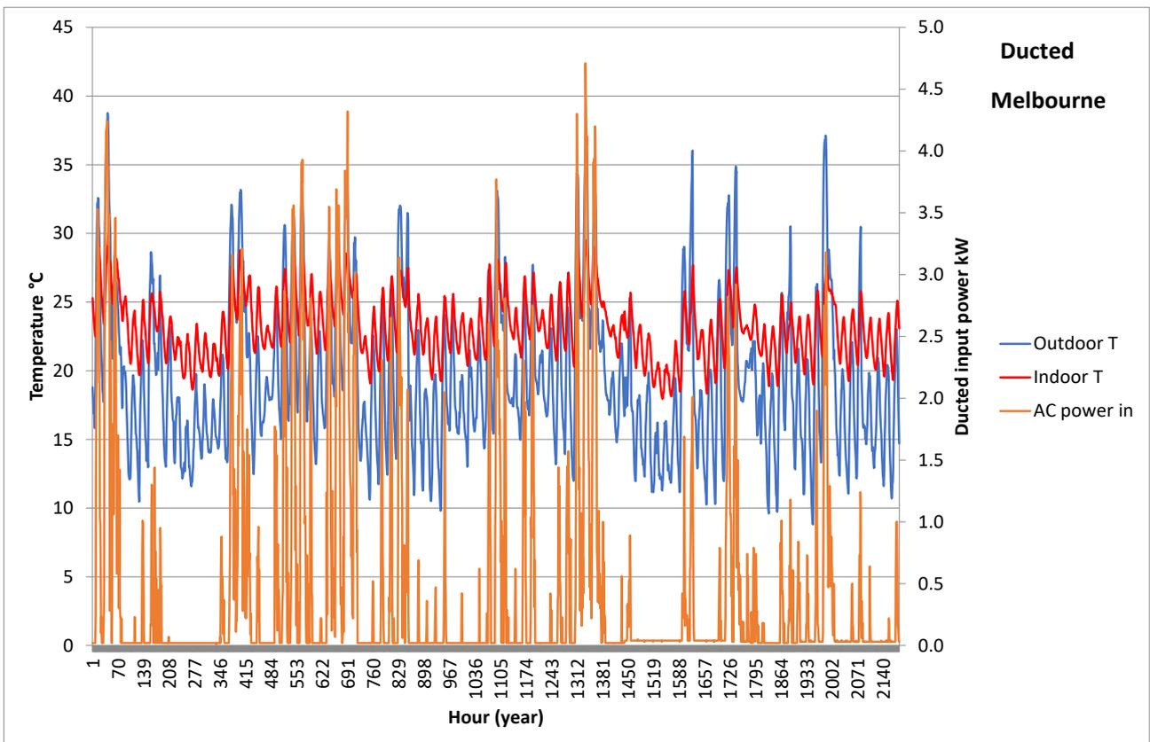
Figure 46: Hourly temperature and ducted power data for Melbourne: Jan, Feb and Dec 2012
