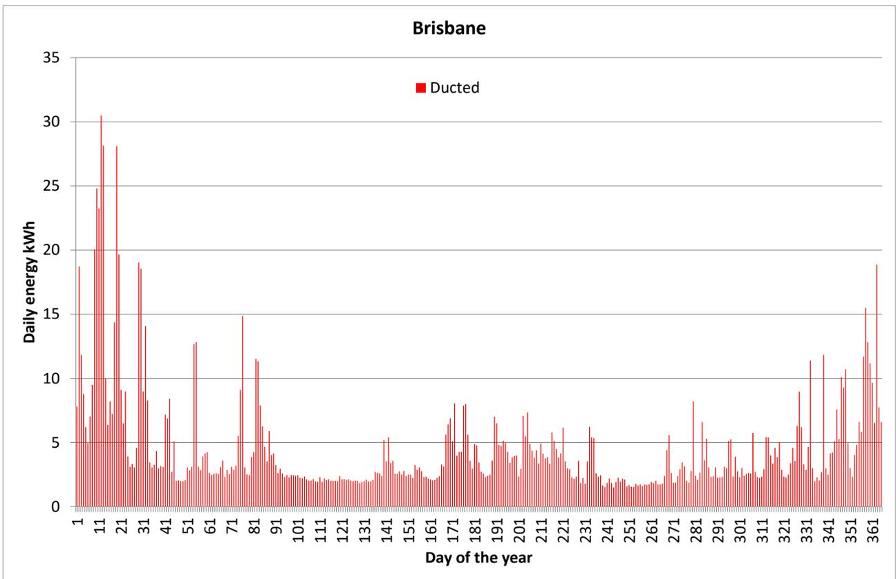
**Figure 43: Daily energy consumption for ducted air conditioners, Brisbane, 2013**
