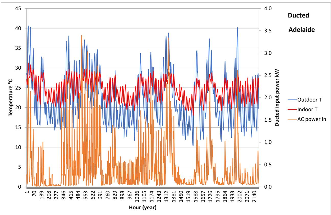
Figure 45: Hourly temperature and ducted power data for Adelaide: Jan, Feb and Dec 2012
