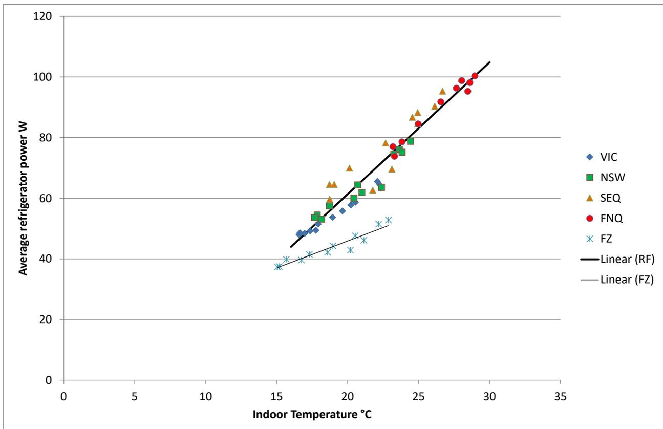
**Figure 71: Model of power versus indoor temperature for household refrigerators and freezers**
