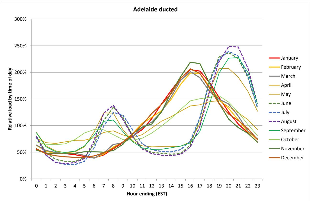
Figure 57: Relative time-of-day profile for ducted air conditioners, Adelaide
