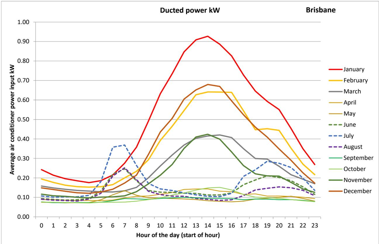
Figure 37: Time-of-day usage for ducted air conditioners by month, Brisbane
