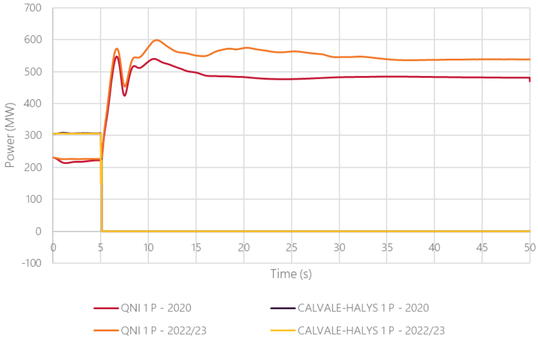
Figure 39 Power flows across key circuits for CQ-SQ non-credible contingency for Case 10 and 2022-23 sensitivity
