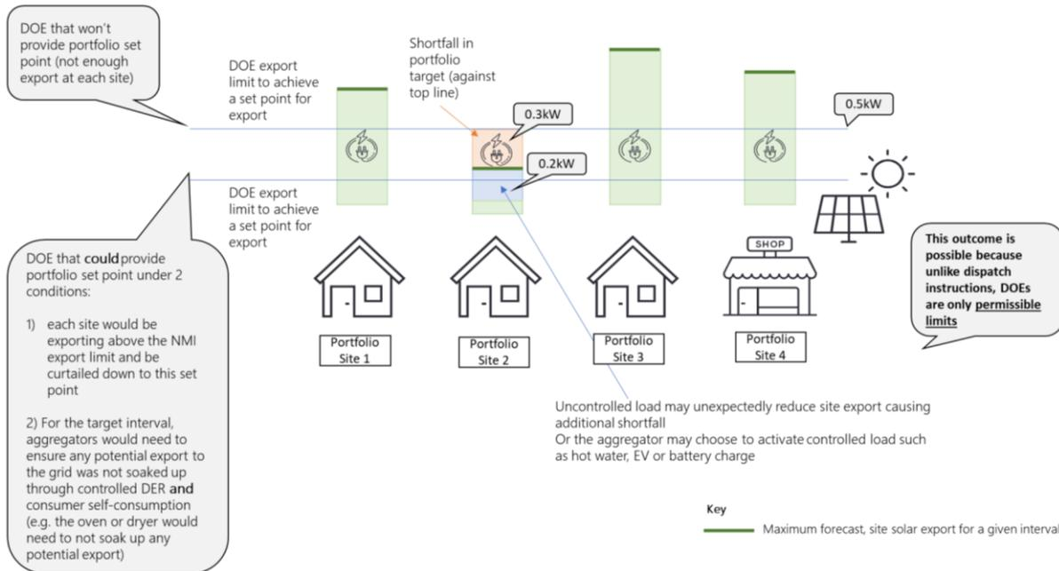
Therefore, DOE limits could provide a firm response across an aggregator portfolio, but are not as reliable as dispatch instructions because they provide operating limits (permissible limits) as opposed to specific directions. The results of the test are illustrated in Figure 9 below, showing the real power (black line) below the upper bound of the DOE limit (blue line). This would require either controlled load to decrease or generation to increase.
