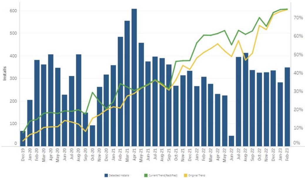
Figure 5 United Energy monthly Volt-VAr compliance assessment
