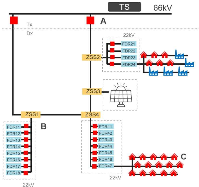
The red boxes and houses represent loads that can be disconnected via UFLS action.
