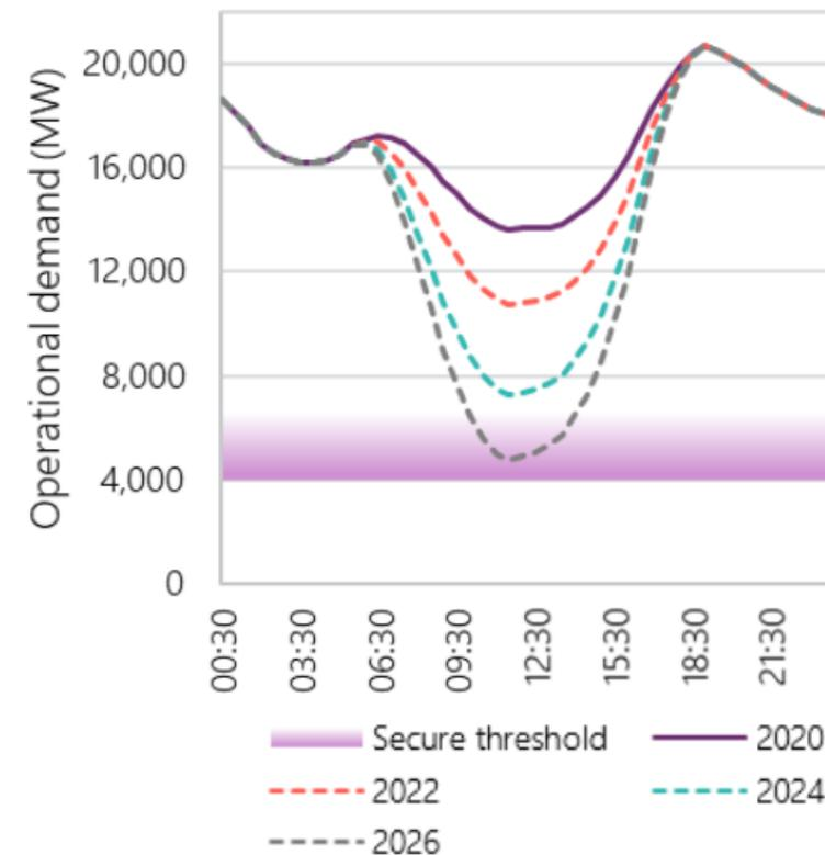
Multiple simulations with varying POE were run to determine the number of hours in which demand fell below 6,000 MW. This represents a wider spread of possibilities than used in Figure 24.
