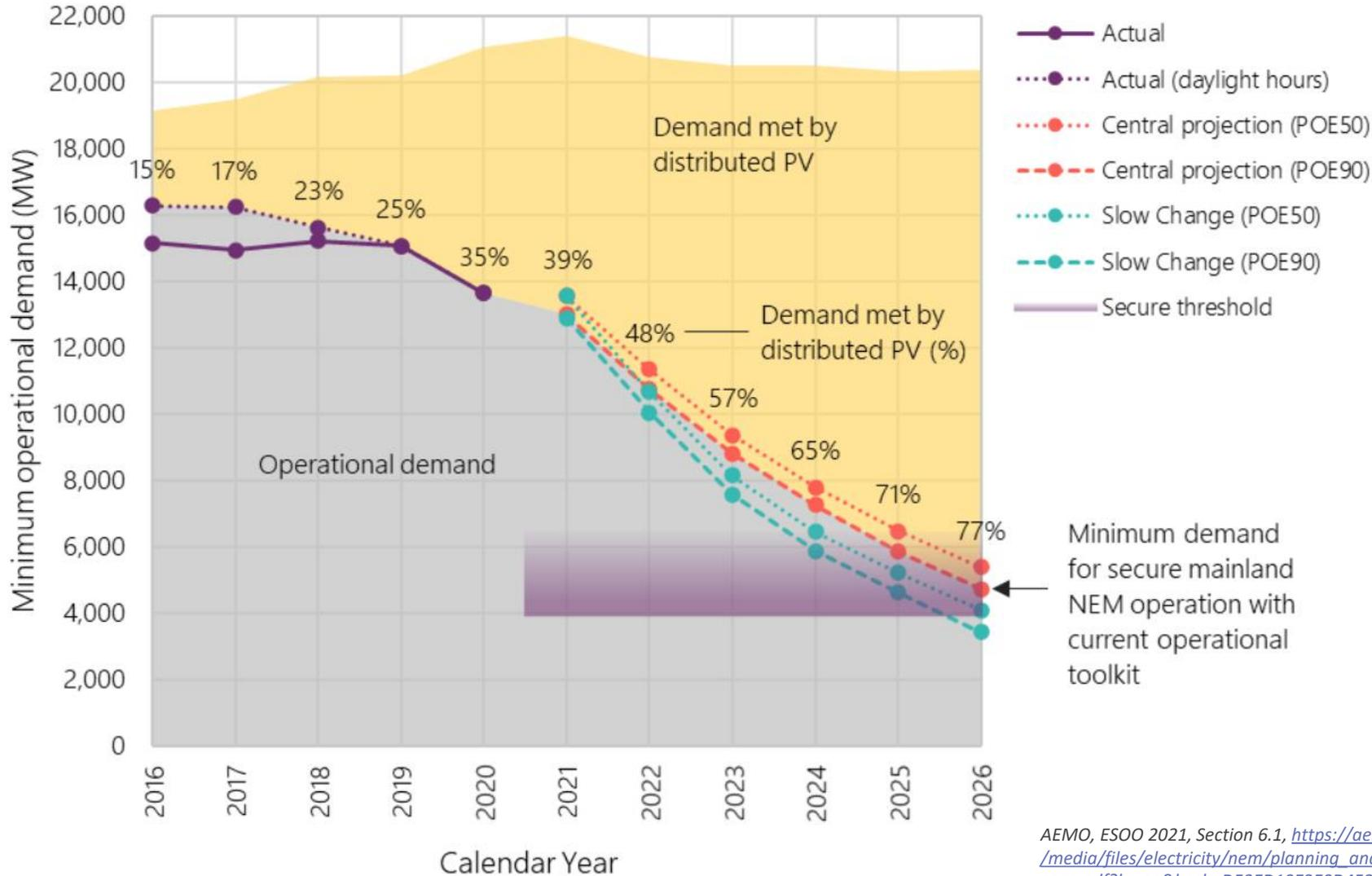
With present operational toolkit, need to maintain a minimum number of synchronous generating units online at all times to provide essential system services:
