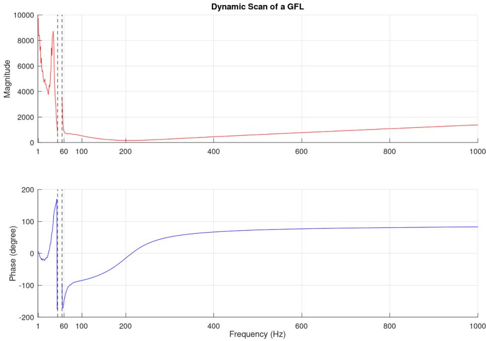
**Figure 11** BESS in GFL mode - Positive sequence scan from 1 to 120 Hz (magnitude and phase) (45 Hz to 55 Hz scan is avoided) (50Hz fundamental frequency)
