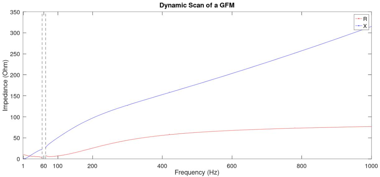
**Figure 13** BESS in GFM mode - Positive sequence scan from 1 to 120 Hz (R and X) (55 Hz to 65 Hz scan is avoided) (60Hz fundamental frequency)
