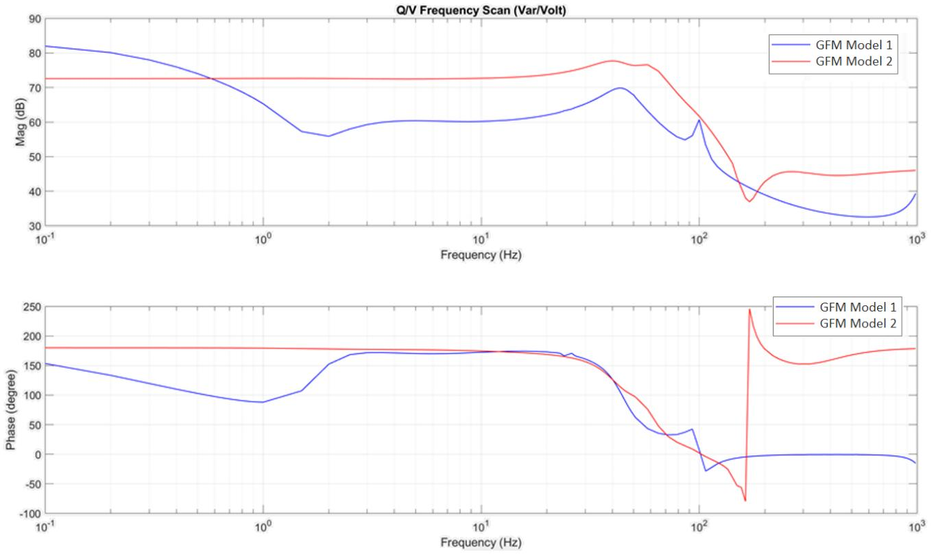
Figure 33 Q/V Impedance Scan - Experimental Scans<sup>28</sup>
