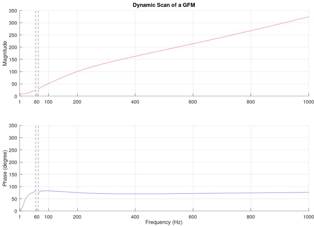
**Figure 15** BESS in GFM mode - Positive sequence scan from 1 to 120 Hz (magnitude and phase) (55 Hz to 65 Hz scan is avoided) (60Hz fundamental frequency)
