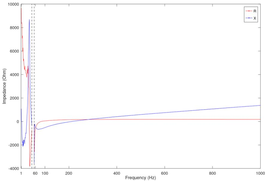
**Figure 9 BESS in GFL mode - Positive sequence scan from 1 to 120 Hz (R and X) (45 Hz to 55 Hz scan is avoided) (50Hz fundamental frequency)**
