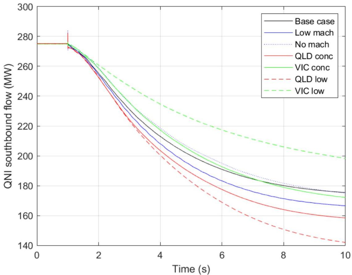
Figure 18 QLD to NSW active power flow response to VIC 363MW load rejection
