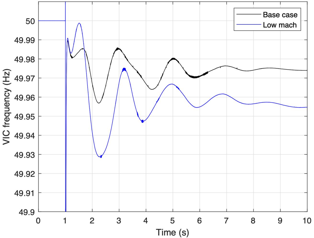
Figure 29 Response of VIC frequency to VIC 100MW generator trip with no GFM plant
