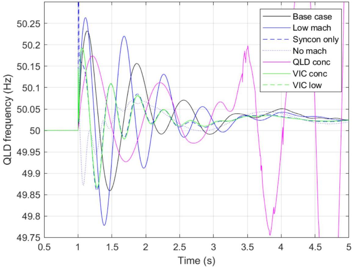
Figure 24 Response of QLD frequency to QLD-NSW separation event
