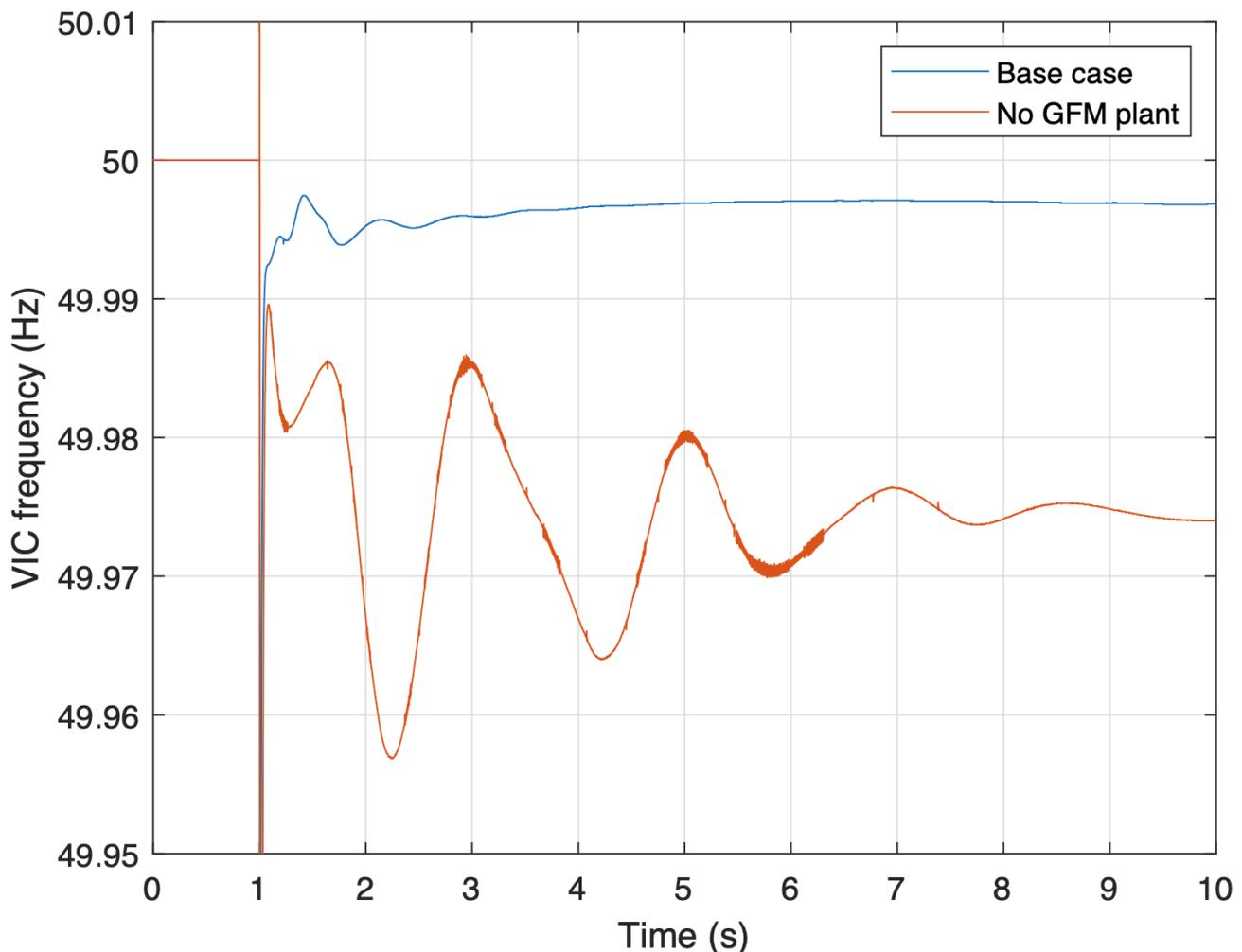
Figure 28 Comparison of base Case 3 for 100MW VIC generator trip with and without GFM plant
