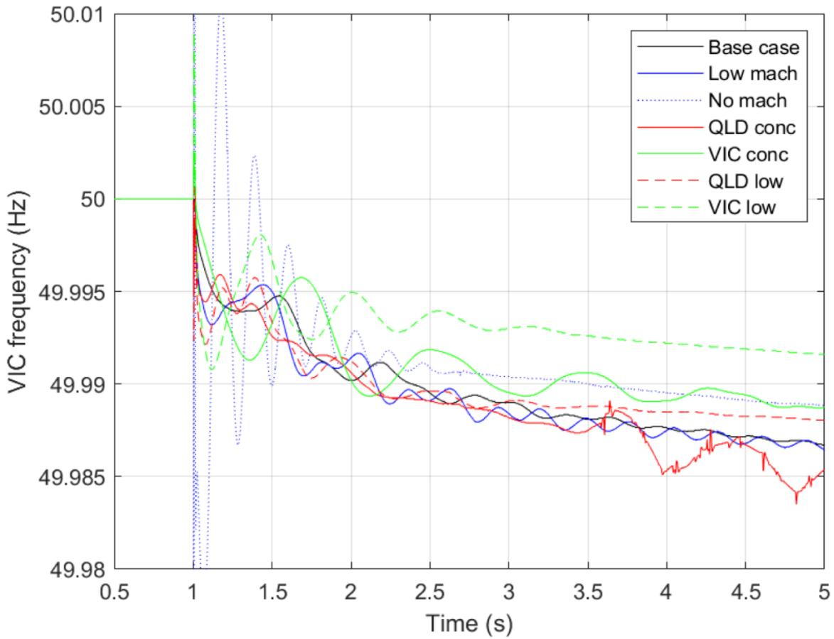
Figure 11 Frequency response in VIC to QLD 600MW generator loss
