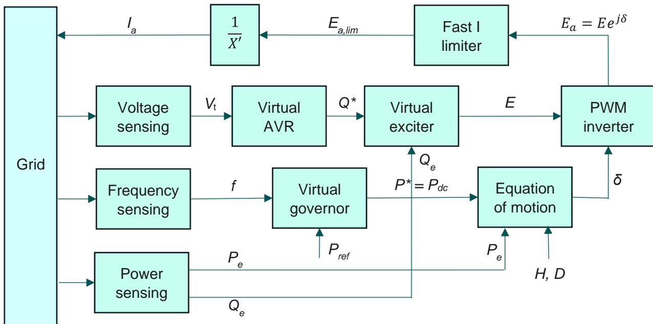
Figure 3 Simplified schematic of generic grid-forming model (VSMINV)
