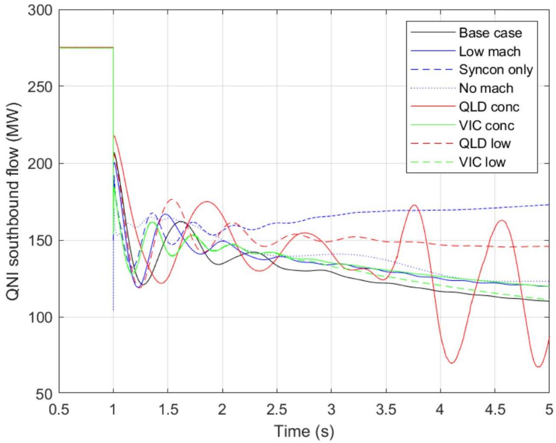
Figure 13 QLD to NSW active power response to QLD 600MW generator loss
