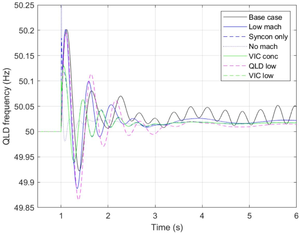
Figure 31 Response of QLD frequency for system separation with additional VIC GFM
