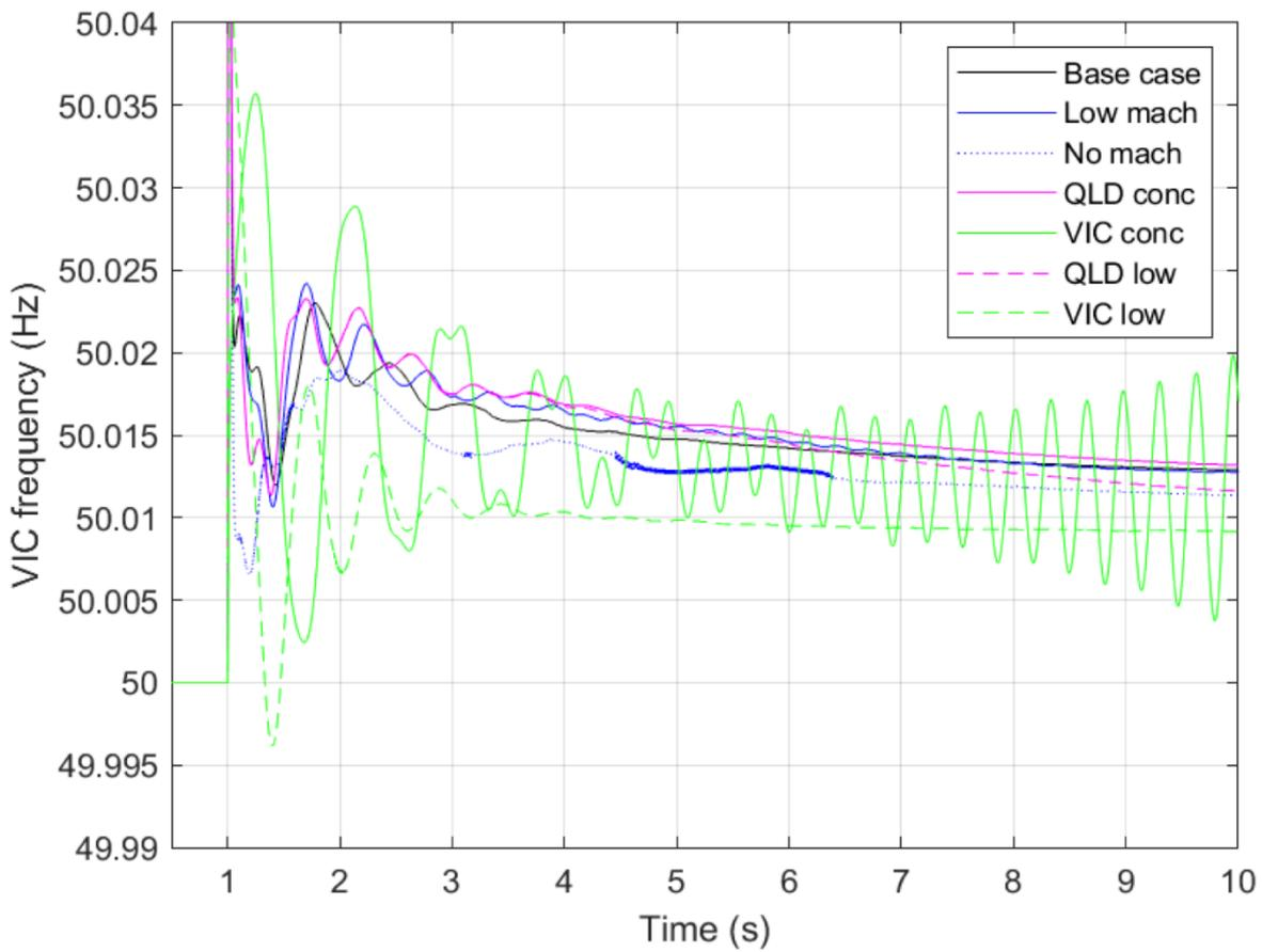
Figure 14 Frequency response in VIC to VIC 363MW load rejection
