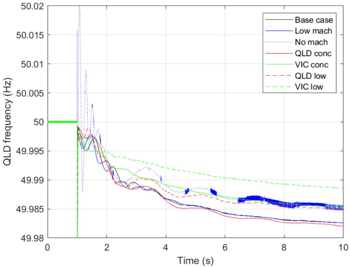
Figure 6 Frequency response in QLD to 500MW VIC generator loss
