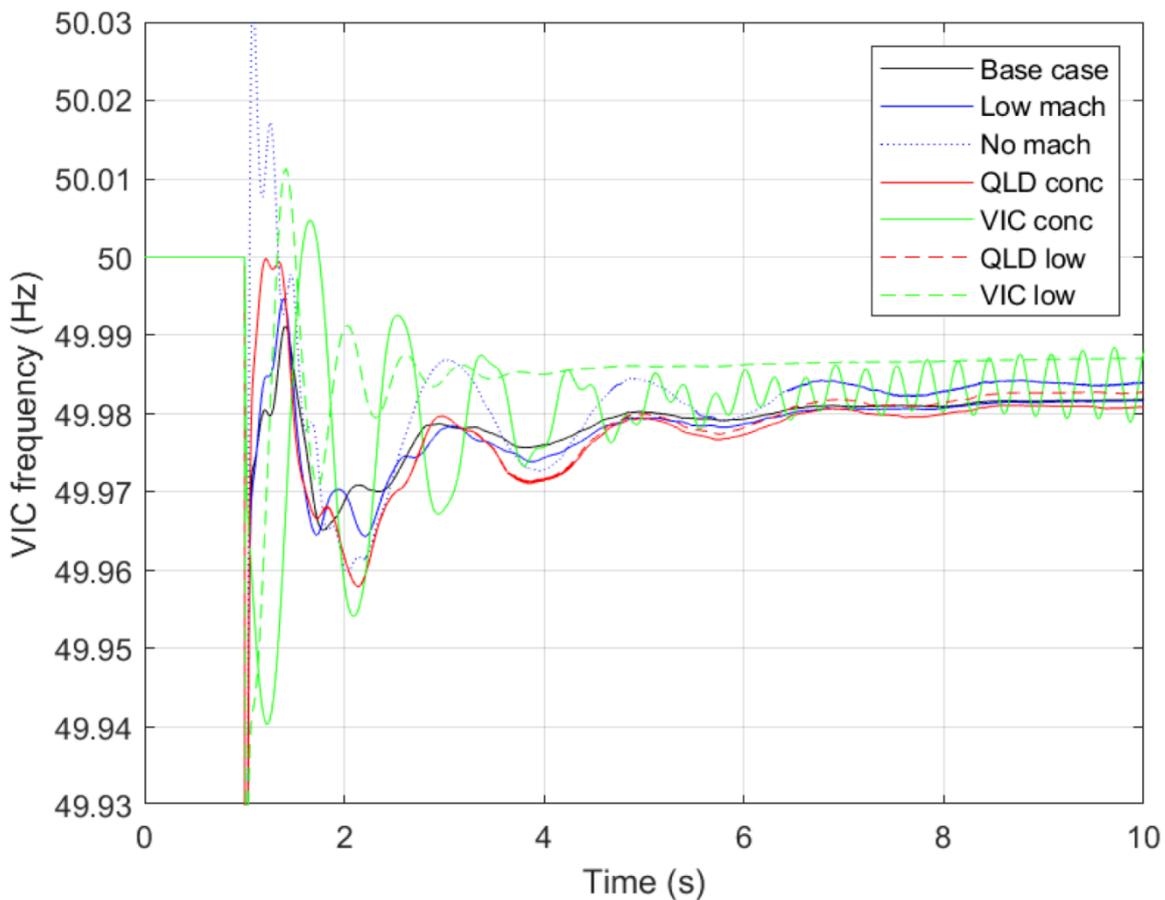
Figure 4 Frequency response in VIC to 500MW VIC generator loss
