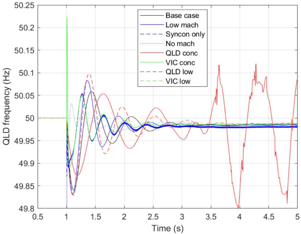
Figure 9 Frequency response in QLD to 600MW QLD generator loss
