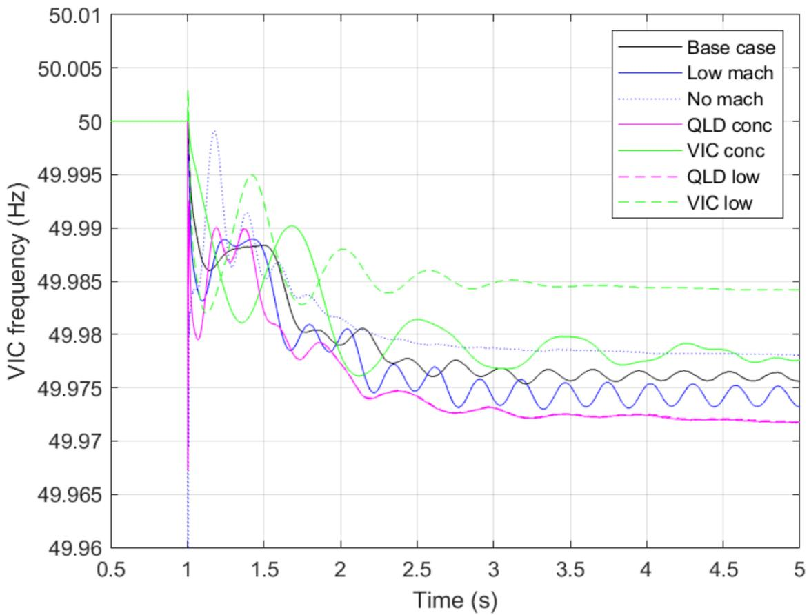
Figure 26 Response of VIC frequency to QLD-NSW separation event
