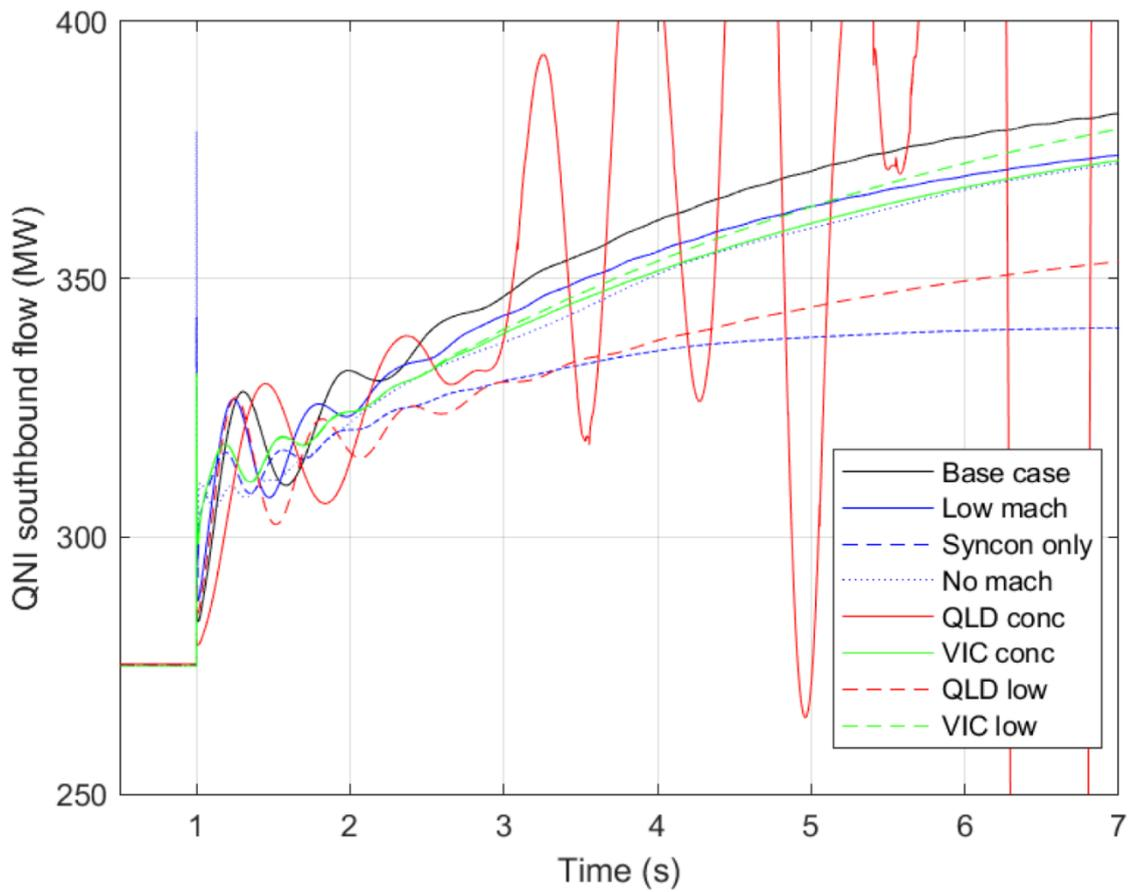
Figure 23 QLD to NSW active power flow response to QLD 400MW load rejection
