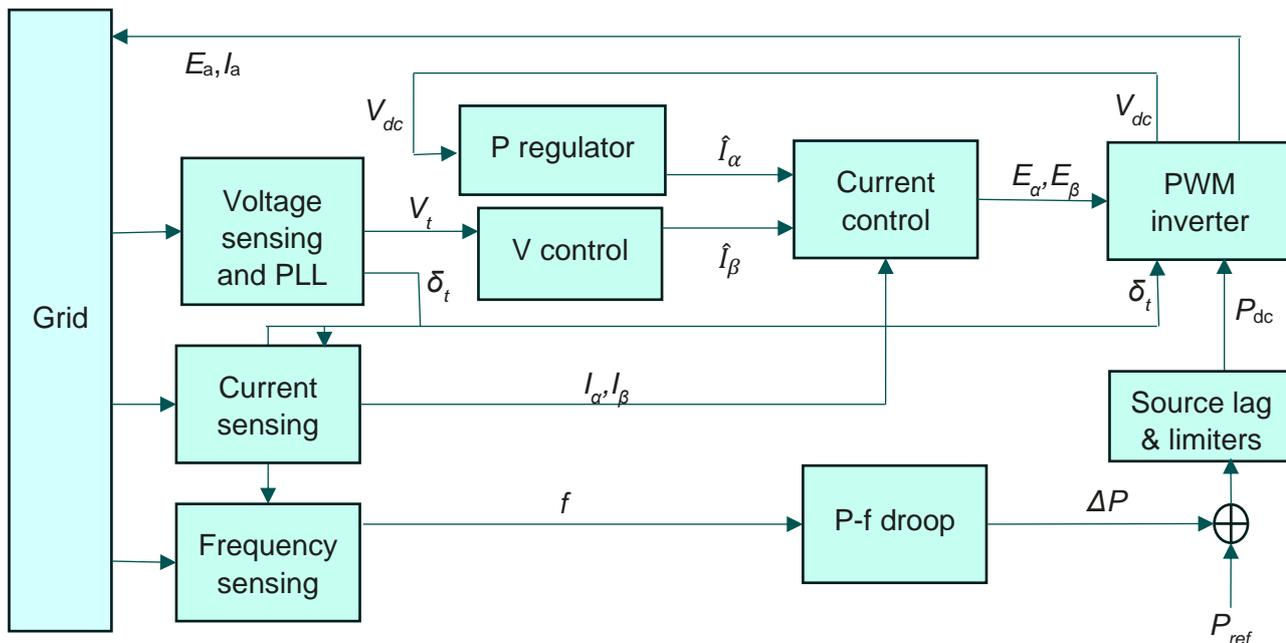
Figure 2 Generic grid-following inverter model (GENINV)
