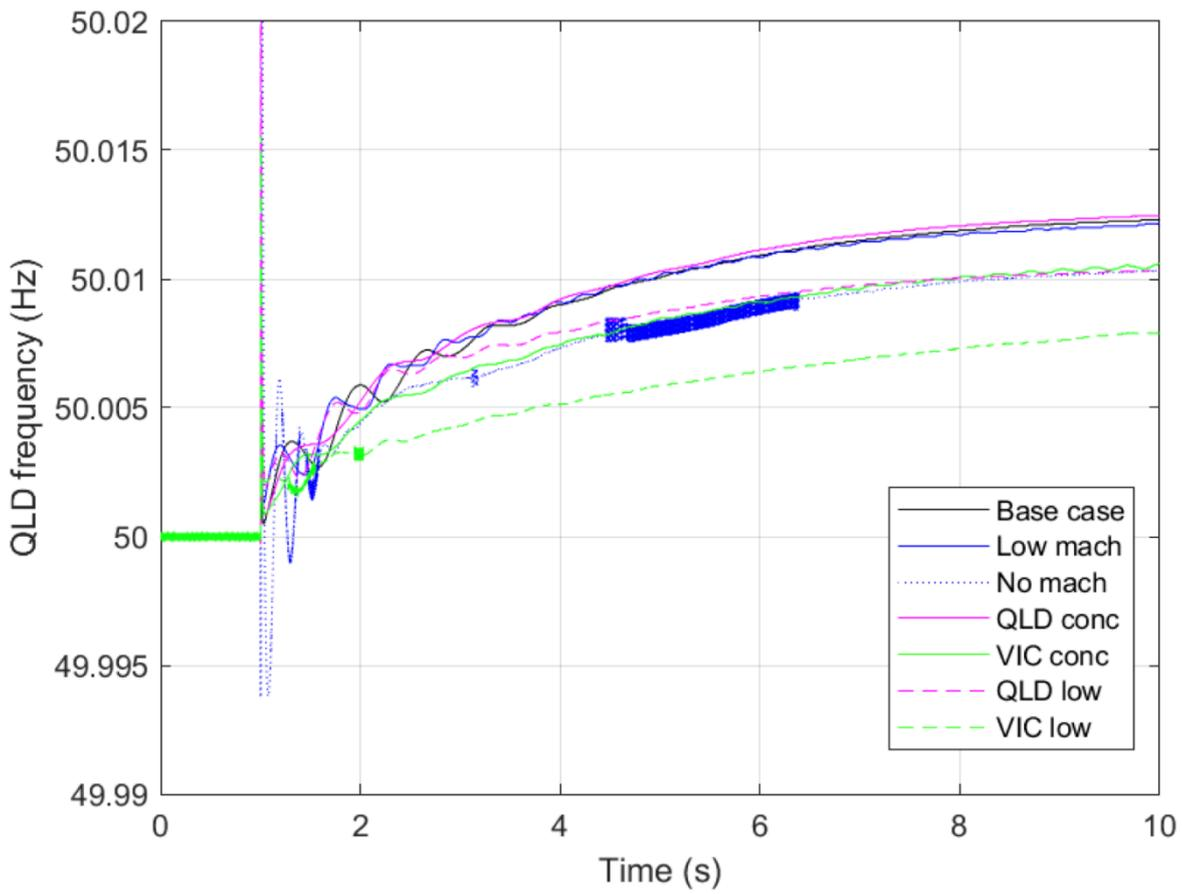
Figure 16 Frequency response in QLD to VIC 363MW load rejection
