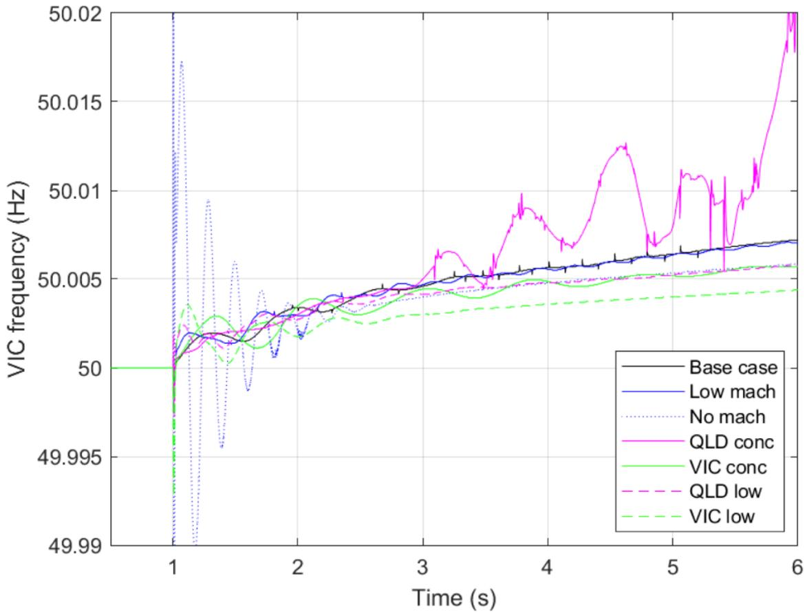
Figure 21 Frequency response in VIC to QLD 400MW load rejection
