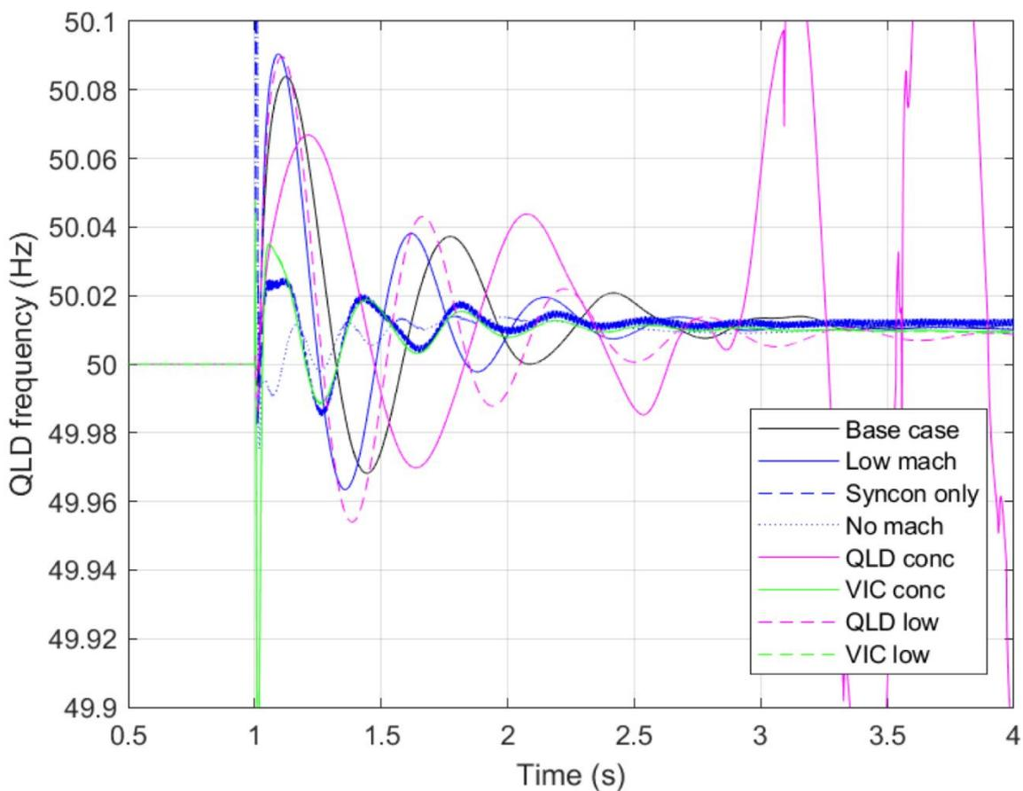
Figure 19 Frequency response in QLD to QLD 400MW load rejection
