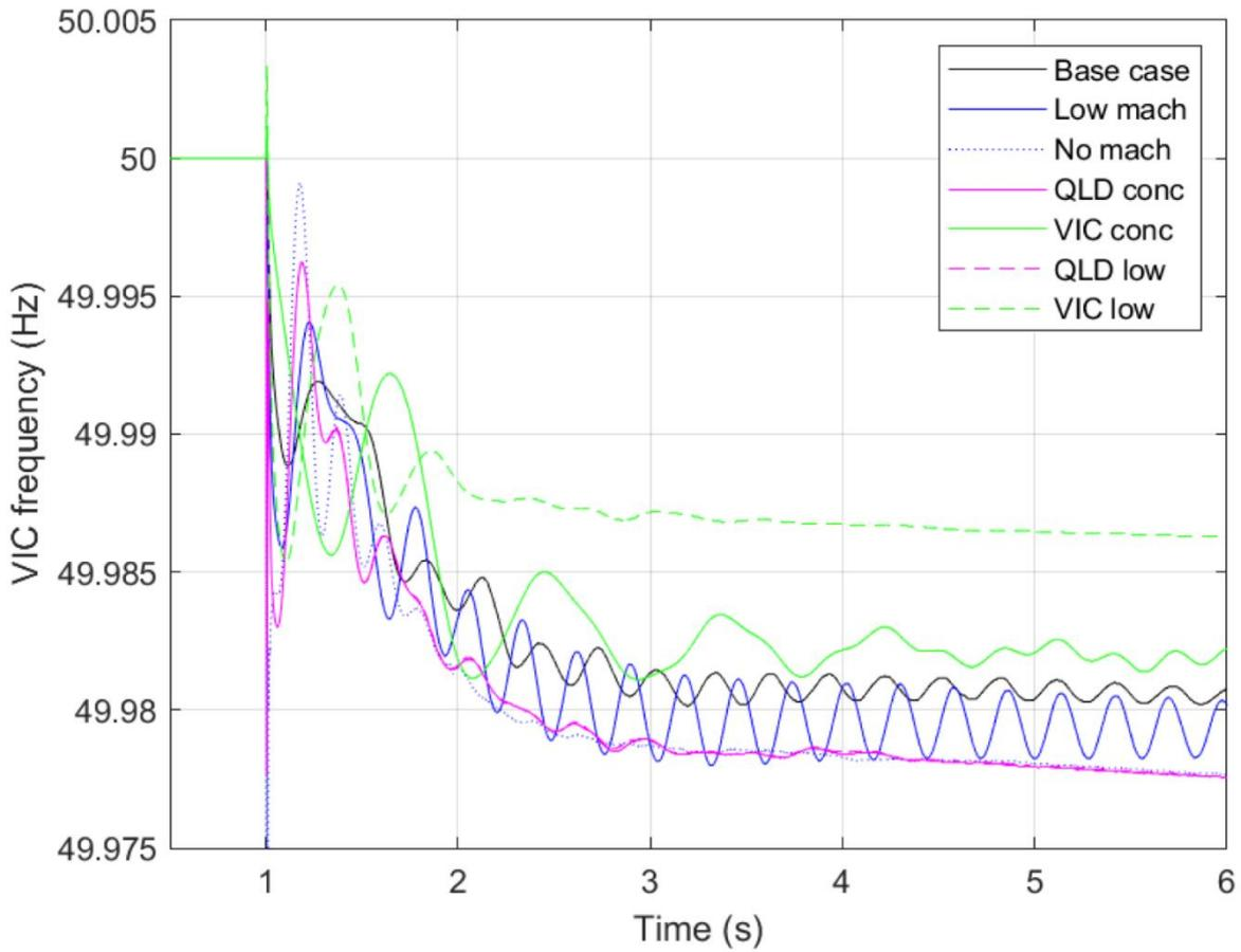
Figure 33 Response of VIC frequency to system separation with additional VIC GFM
