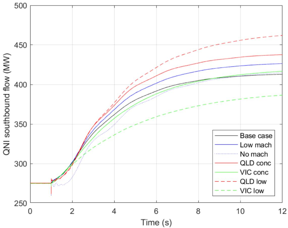
Figure 8 QLD to NSW active power flow response to 500MW VIC generator loss
