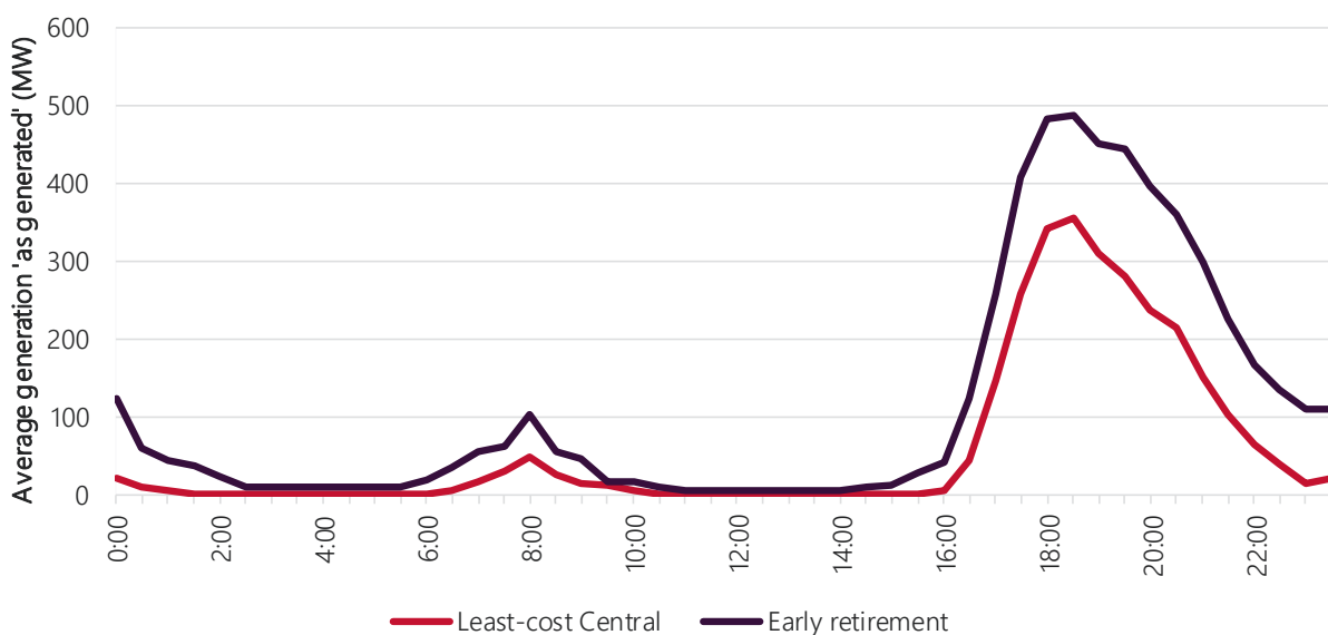
Figure 31 Projected average time-of-day gas generation in Victoria in June 2028 with and without early coal retirement
