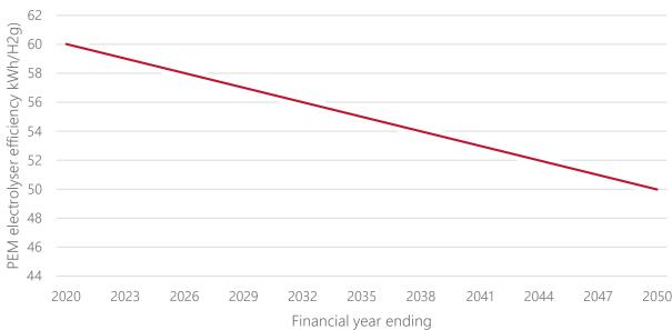
Figure 28 Efficiency projections for PEM electrolysers
