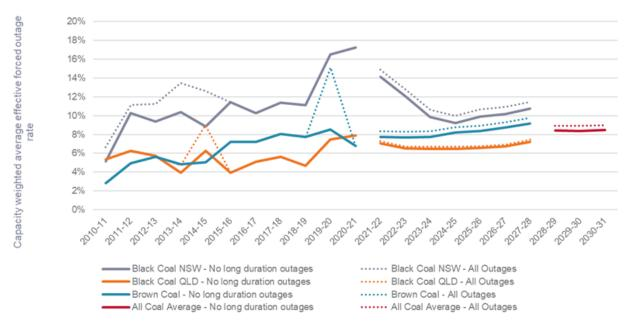
Figure 29 Effective full forced outage rate projections for coal-fired generation technologies
