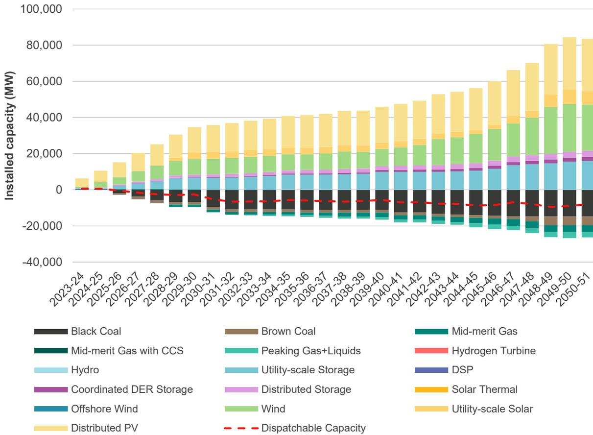
Despite the lack of any explicit decarbonisation objective, Figure 34 below shows that even in the *Slow Change* scenario, the energy mix is dominated by VRE, with over 94% of generation being from renewable sources by 2049-50. By then, the projected mix of VRE generation is 55% wind, 16% utility-scale solar and 29% distributed PV.
