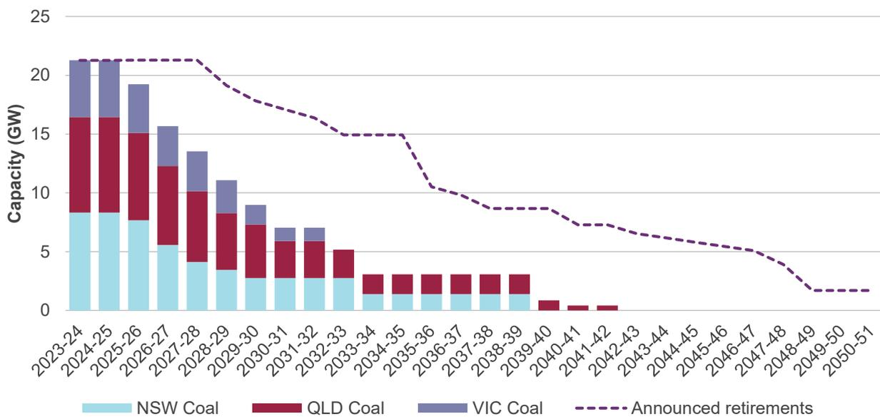
The pace of transformation will be influenced by the availability of transmission to deliver VRE generation to consumers across the planning horizon. Figure 11 demonstrates the faster retirement schedule that would be required if transmission expansion was not part of AEMO’s ODP.
