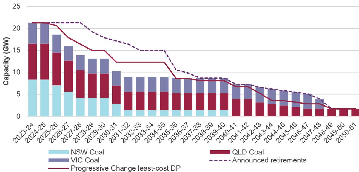
Figure 33 below shows the development of capacity in the *Slow Change* scenario. Policy-driven developments and earlier coal closures slow in the 2030s, as the policies are met. In the longer term, less electrification of other sectors leads to more muted generation investment, although additional VRE development, complemented by energy storage, is developed to replace end of life coal retirements.
