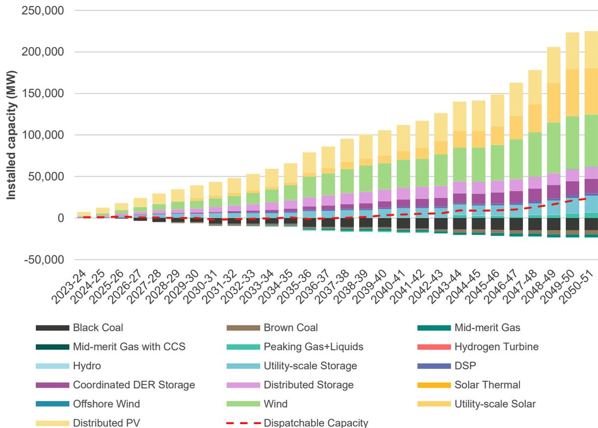
In terms of energy production, Figure 17 demonstrates the forecast change in the energy mix that is very different to today's energy system, both technologically and geographically. Renewable energy is forecast to expand to approximately 93% of energy generated by 2049-50. The projected mix of VRE by 2049-50 is
