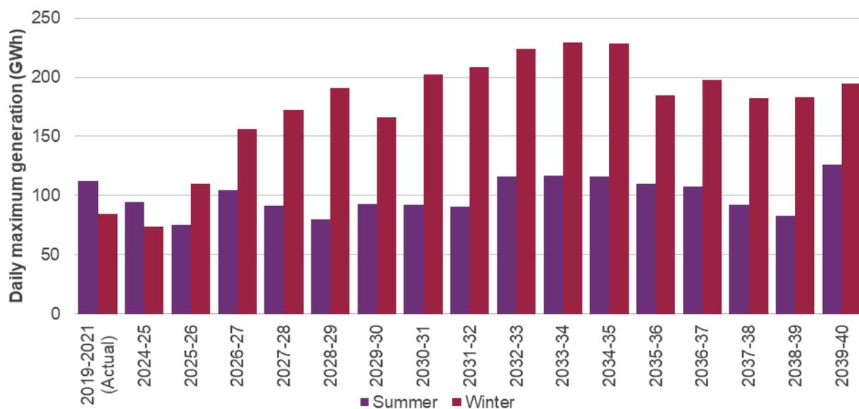
As coal capacity declines, gas generators are projected to start more frequently and run for longer periods of time (as seen in Figure 24 below), depending on the investments made in energy storage – more so, if coal generators cannot operate as flexibly as assumed for sustained periods.
