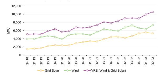
Figure 47 Record high instantaneous wind and combined VRE output in Q2 2022 Maximum quarterly instantaneous generation by fuel type
