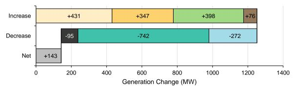
Distributed PV Grid Solar Wind Black Coal Brown Coal Gas Hydro Net
