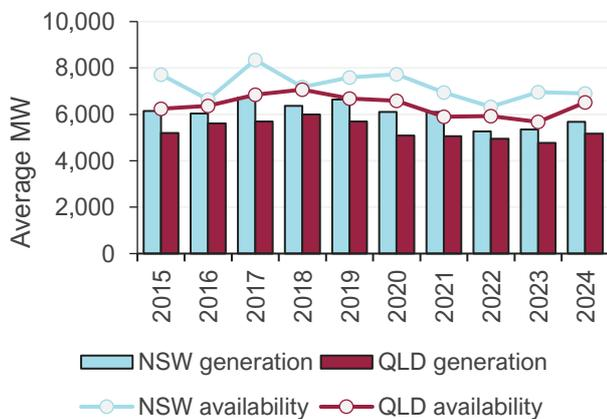
**Figure 32 Significant decrease in Queensland coal-fired capacity on outage**
