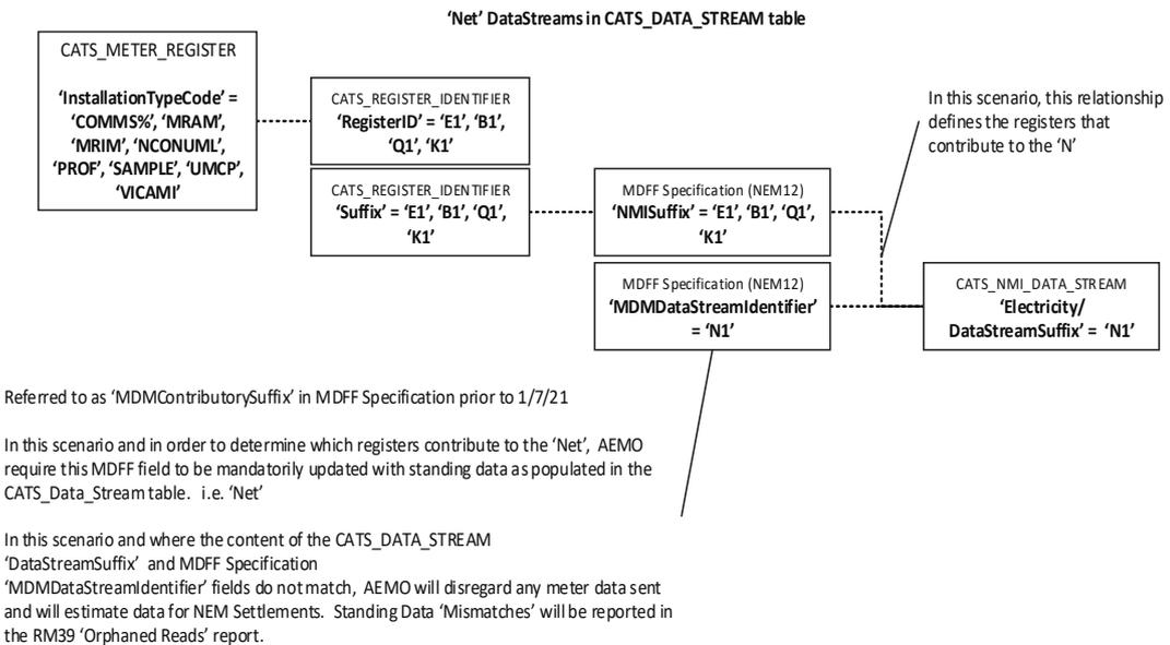
Example of an Interval Meter “Suffix” – Register Level DataStreams
