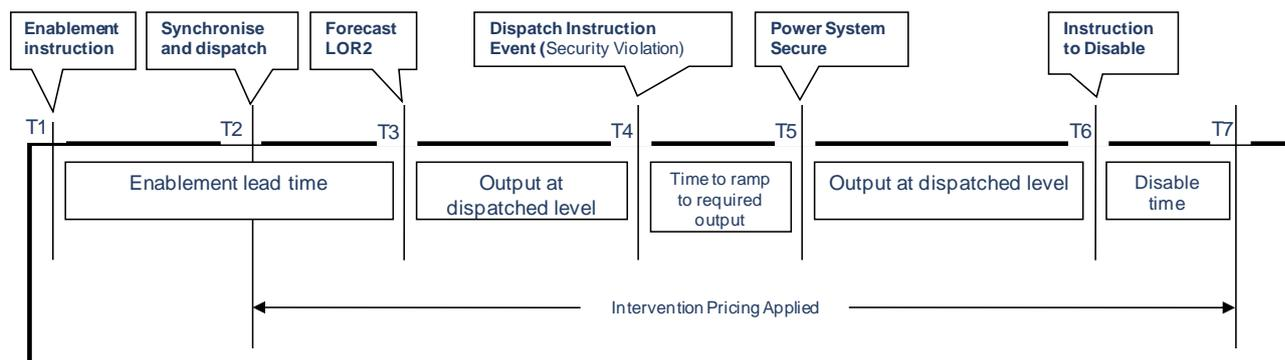
Enablement means preparing the *reserve equipment* to be *dispatched*. For example, Figure 1 demonstrates a fast response generator that does not need to be synchronised at the forecast LOR2 time (T2) to provide the reserve capacity. Note: a slow response generator may require *synchronising* and *loading* to its *minimum operating level* or some nominated level at the start of the LOR2 period (as shown in Figure 2), so that it can provide the reserve capacity within the timeframe required.
