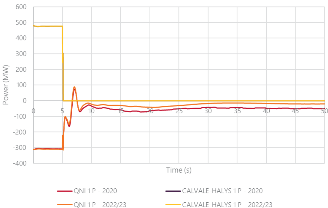
Figure 36 Power flows across key circuits for CQ-SQ non-credible contingency for case 3 and 2022-23 sensitivity
