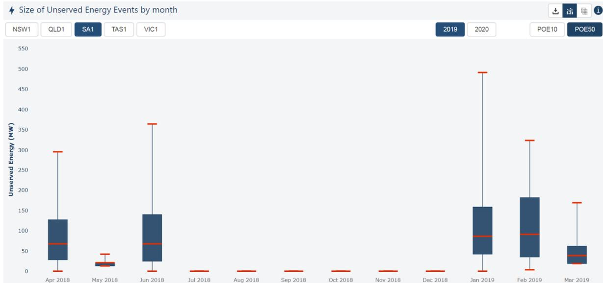
Figure 12 gives more detailed insight into the USE observed through modelling outcomes by considering the frequency of events as well as the expected size of the USE events. The chart shows the 10% POE condition's USE events are larger in size and more frequent than those of the 50% POE condition.
