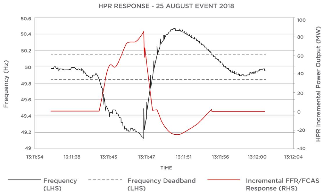
HPR currently provides its 'premium' fast-frequency capability through participation in the existing contingency FCAS markets, albeit with a much faster response than required by these markets. Recognising that batteries are already providing a form of Fast Frequency Response, we are also working closely with relevant parties at ESB, AEMO and ESB in exploring appropriate incentives to value fast frequency services.
