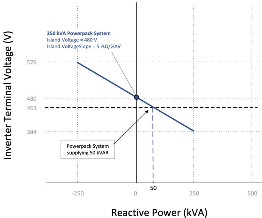
Figure 2 – Voltage Forming Mode – Real Power
