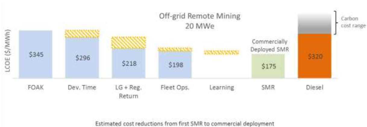
Figure 9: A bridge diagram for off-grid mining. Development time and cost becomes a material economic driver and is a requirement from industry to be less than 6 years. We expect a commercially deployed SMR to be competitive to the diesel benchmark without a price on carbon.
