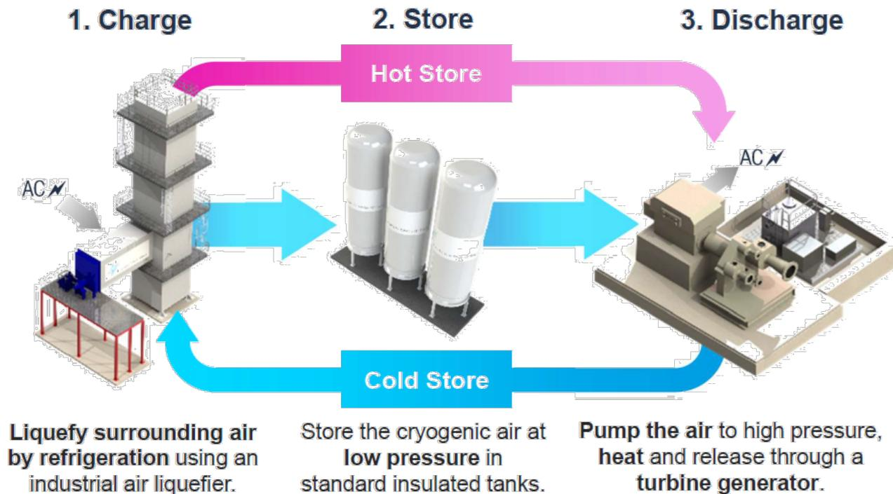
Additional **hot** and **cold** thermal recycling increases efficiency
