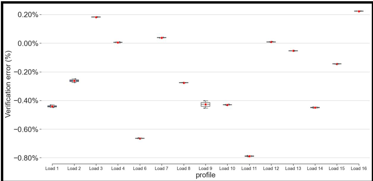
Figure 3.3. Error distribution of 50ms sampling rate for different switched response profiles, 1s service.
