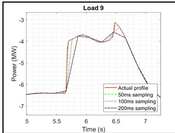
Figure 3.6. Response shape with different sampling rates for load 9
