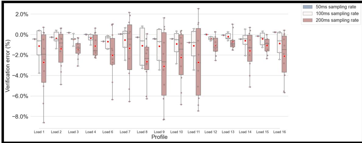
Figure 3.4. Error distribution of different sampling rates for all switched response profiles, 1s service.
