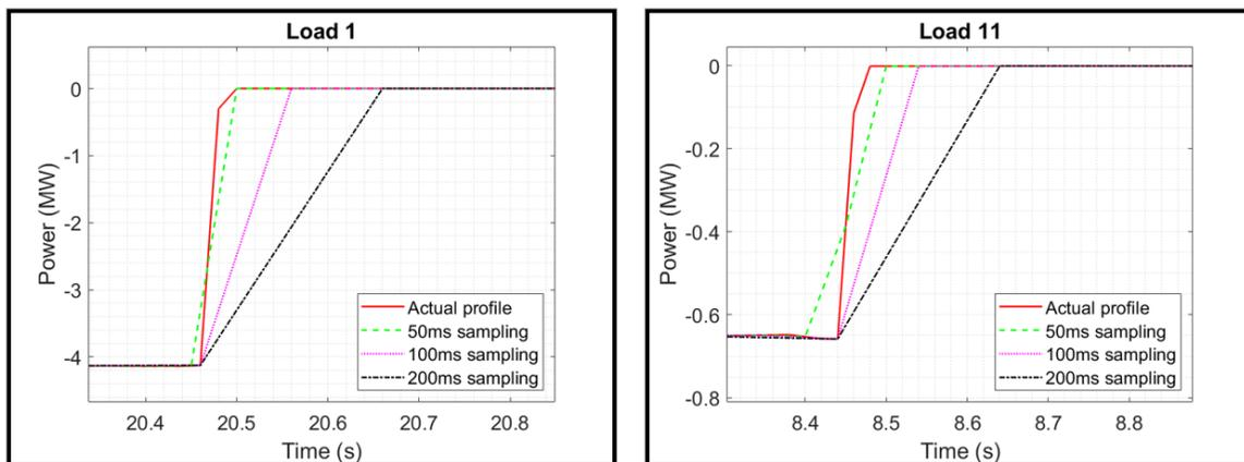
Figure 3.5. Response shape with different sampling rates for loads 1 and 11
