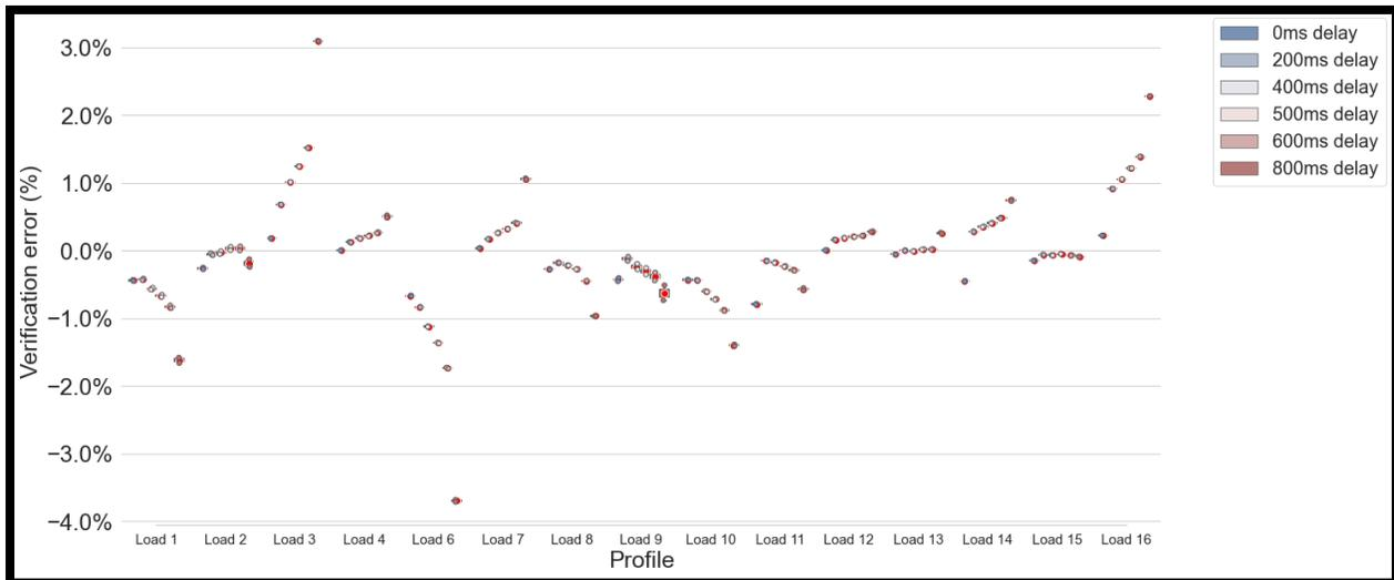
Figure 3.11. Assessment errors for 50ms sampling rate considering different values of delays in the response
