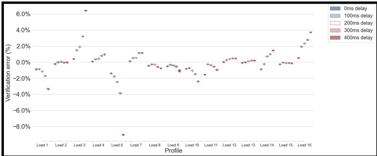
Figure 4.7. Assessment errors for 50ms sampling rate considering different values of delays in the response, 0.5s service
