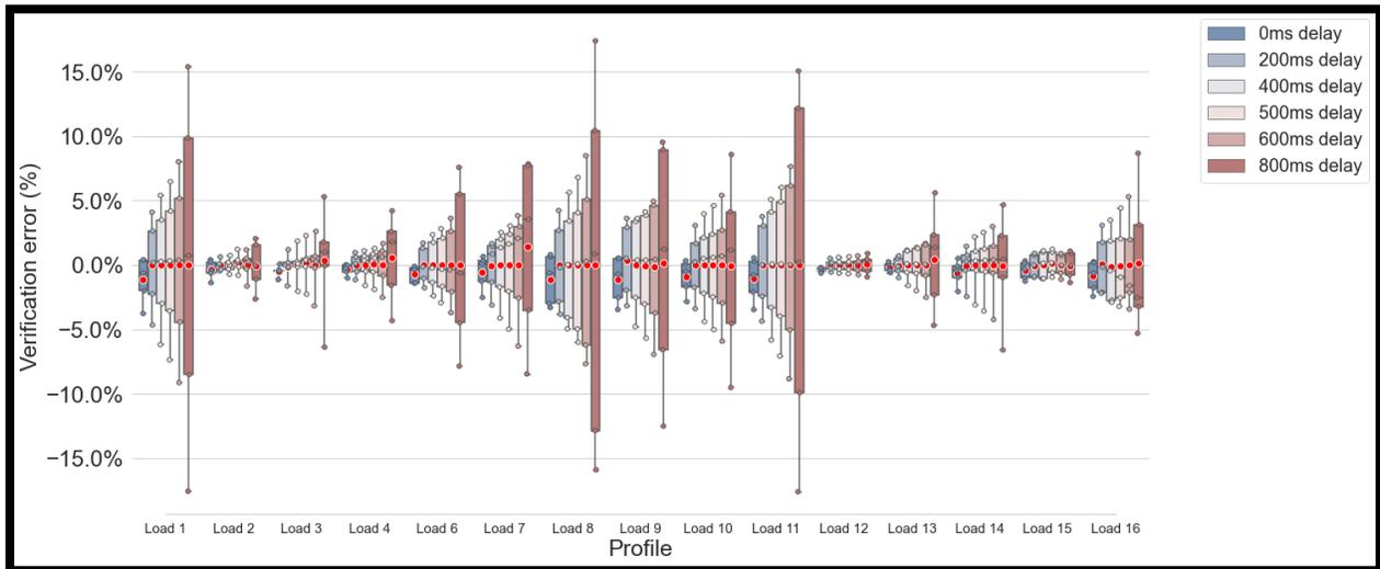
Figure 3.10. Assessment errors for **100ms** sampling rate considering different values of delays in the response
