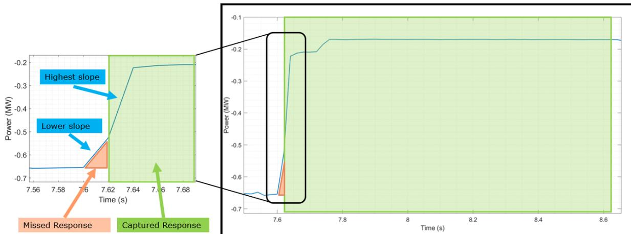
Figure 2.3. Visual representation of the rolling assessment window in capturing a switched response
