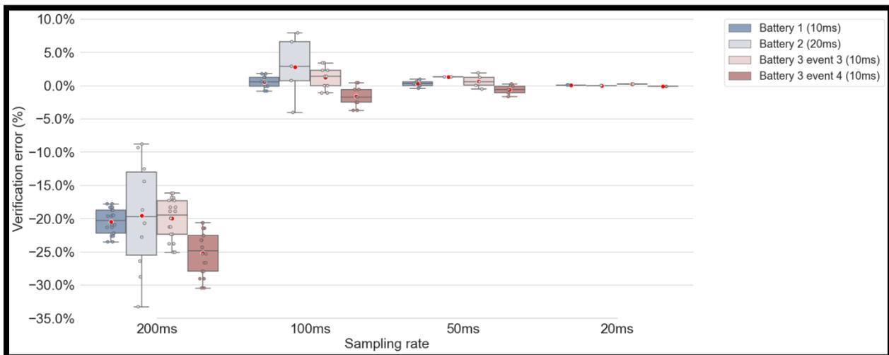
Figure 4.8 Error distribution of lower sampling rates for batteries in the assessment case based on FDT considering 0.5s service
