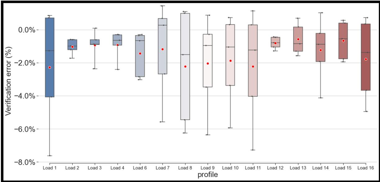
Figure 4.2 Error distribution of 100ms sampling rate for different switched response profiles, 0.5s service.
