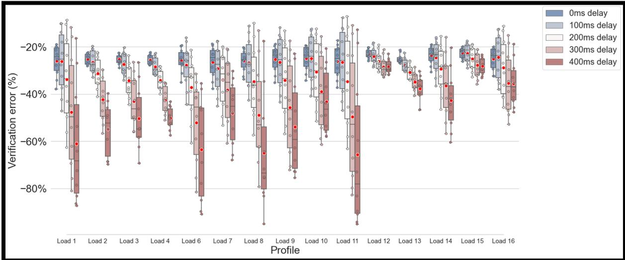
Figure 4.5 Assessment errors for **200ms** sampling rate considering different values of delays in the response, 0.5s service
