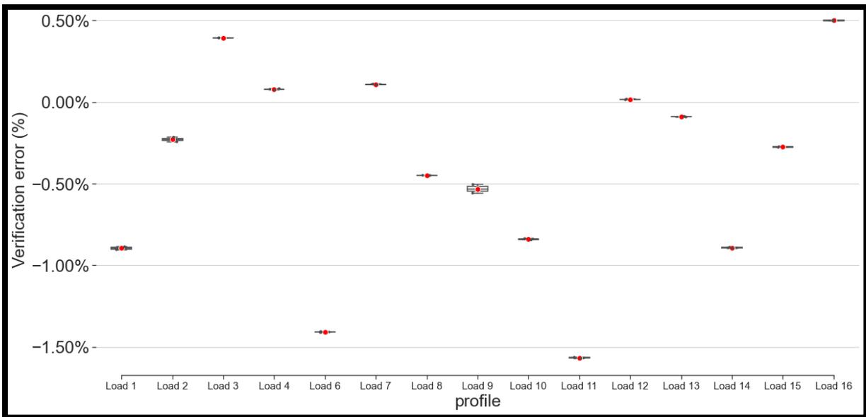
Figure 4.3 Error distribution of 50ms sampling rate for different switched response profiles, 0.5s service.
