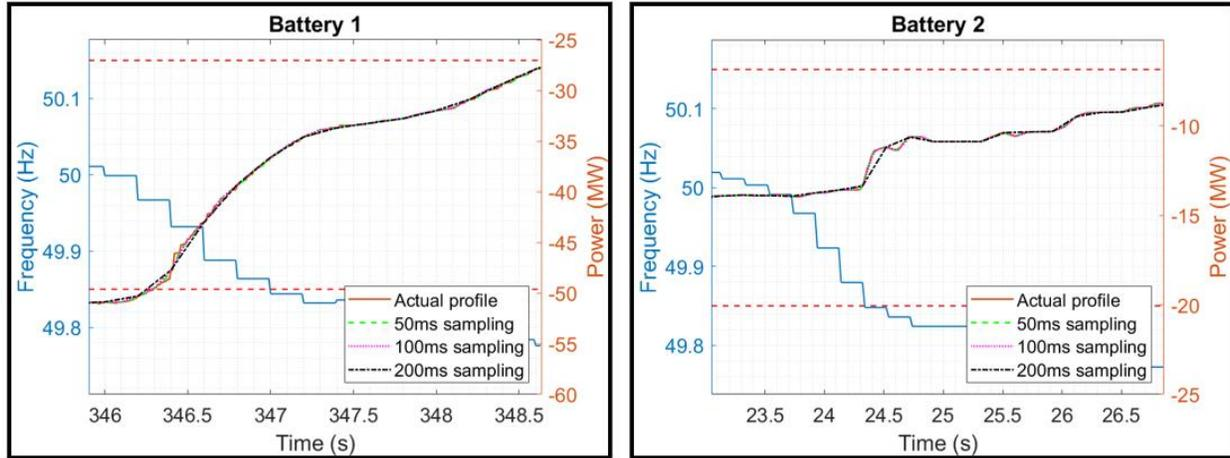
Figure 3.13. Response shape with different sampling rates for Battery 1 and Battery 2
