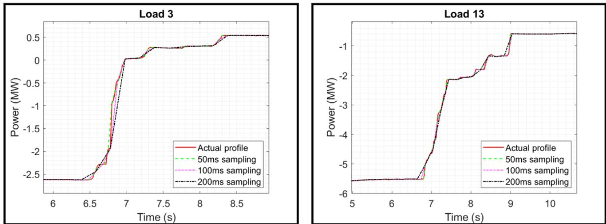
Figure 3.7. Response shape with different sampling rates for loads 3 and 13
