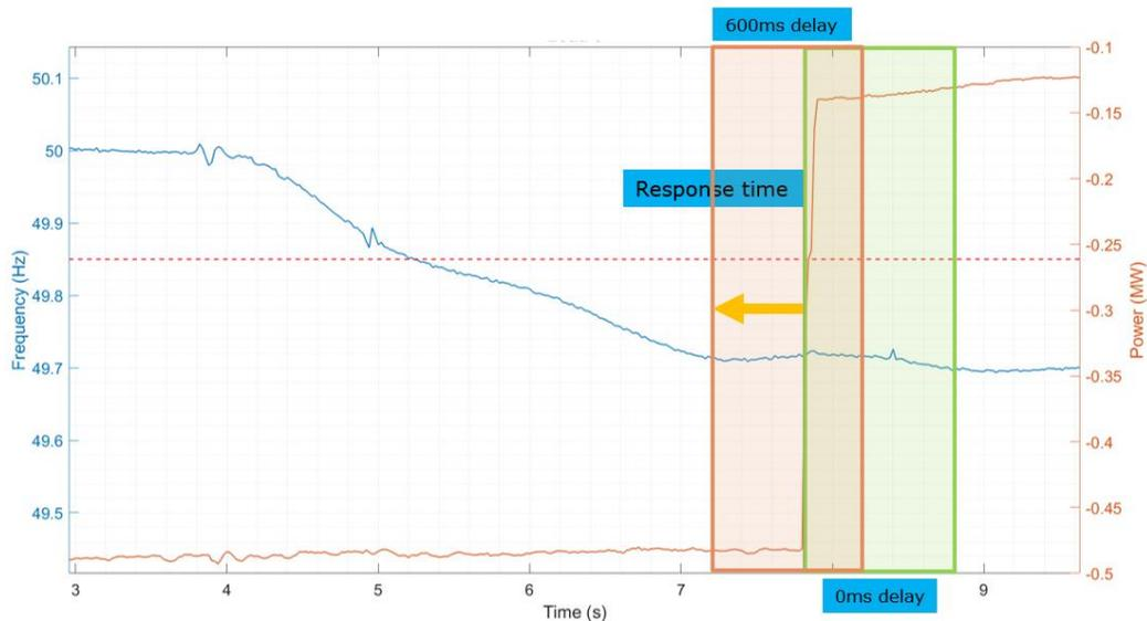
Figure 3.8. Considering a response delay of 600ms for a switched load based on the rolling assessment window
