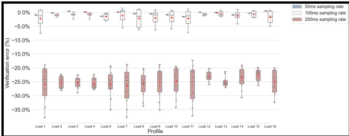
Figure 4.4 Error distribution of different sampling rates for all switched response profiles, 0.5s service.
