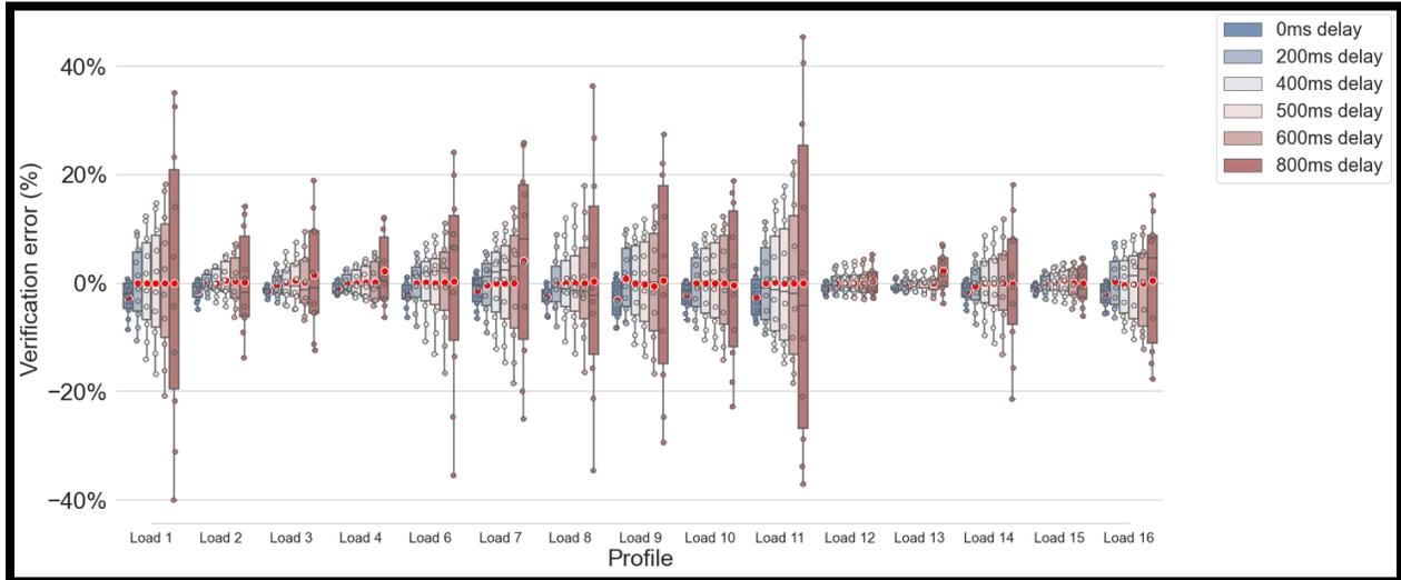
Figure 3.9. Assessment errors for **200ms** sampling rate considering different values of delays in the response
