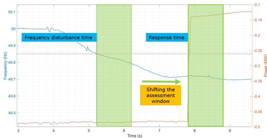
Figure 2.2. Shifting the starting point of the assessment window to the “most plausible” response time
