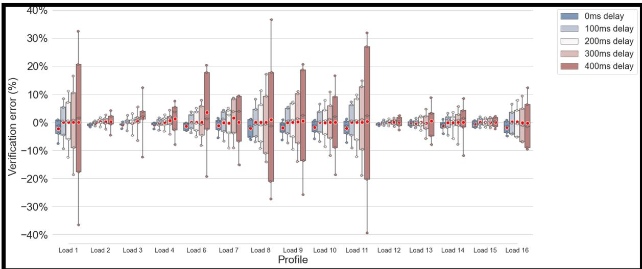
Figure 4.6 Assessment errors for **100ms** sampling rate considering different values of delays in the response, 0.5s service
