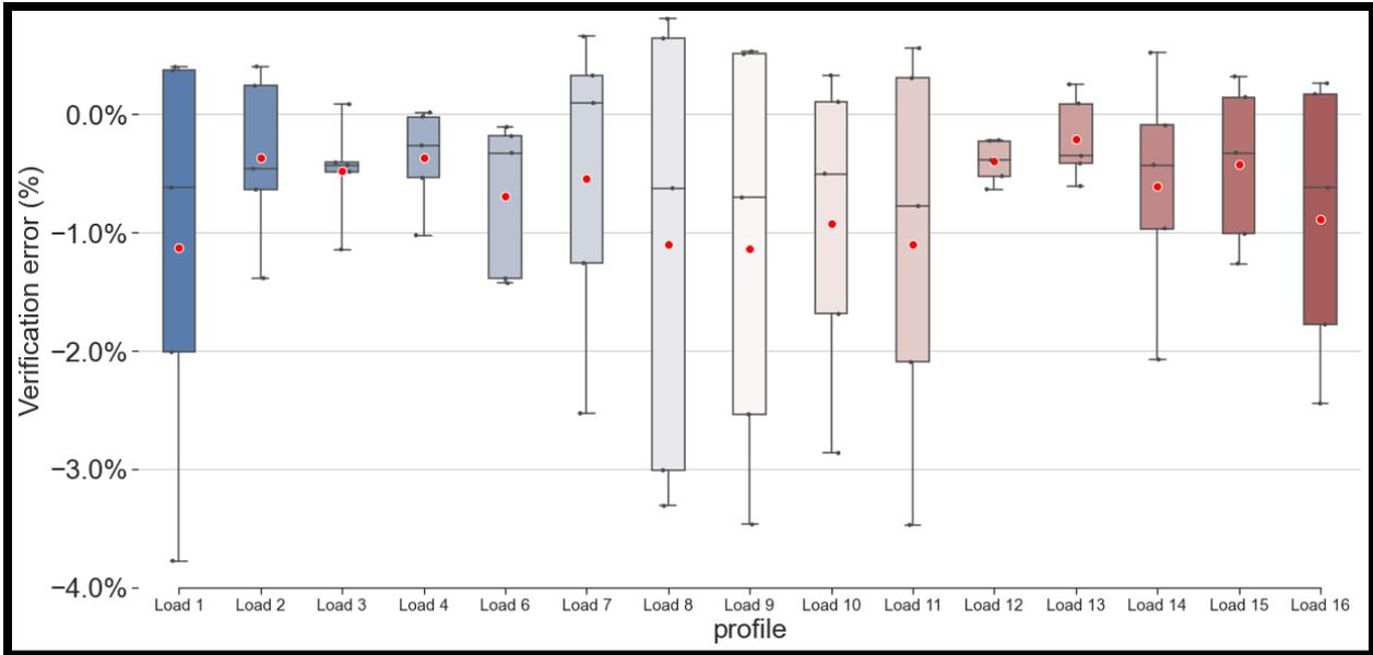
Figure 3.2. Error distribution of 100ms sampling rate for different switched response profiles, 1s service.
