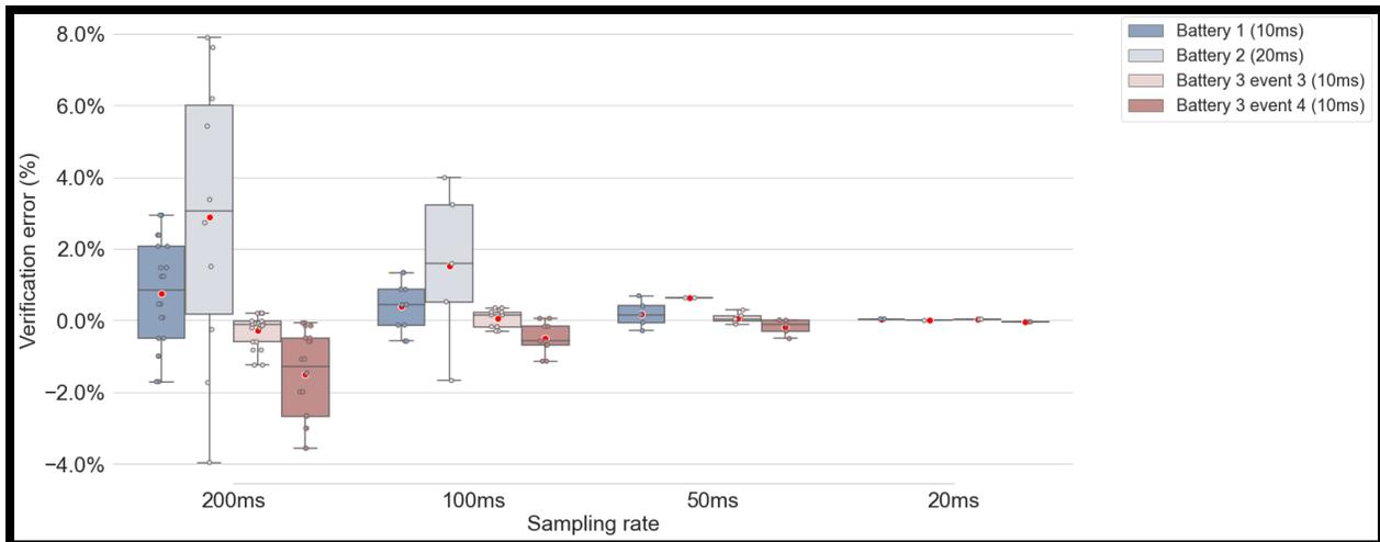
Figure 3.12. Error distribution of lower sampling rates for batteries in the assessment case based on FDT
