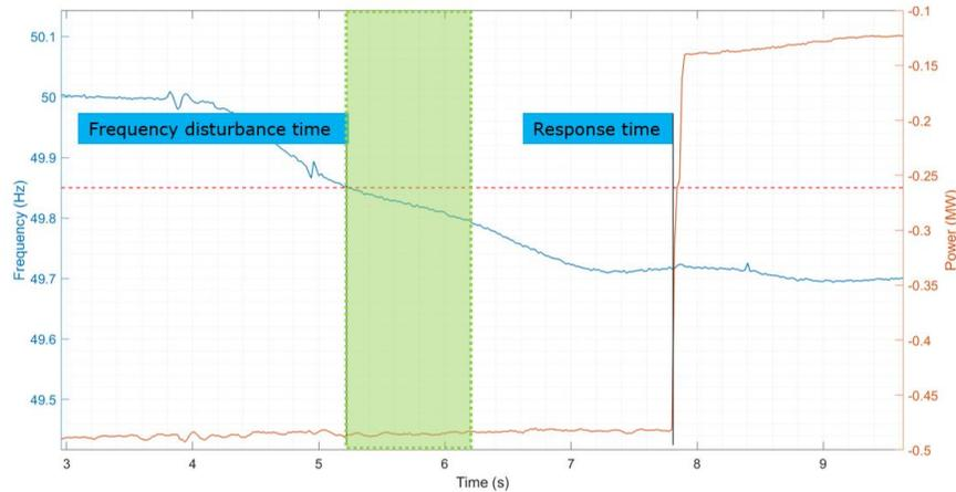
Figure 2.1. Example of frequency and active power profiles for a switched load, with relevant response delay window
