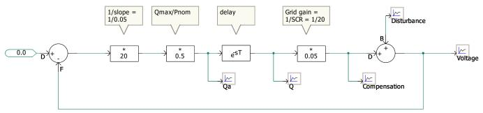
It is important to note that the above system performance can be investigated based on the angle which is defined between Voltage and Compensation (and not between Disturbance and Compensation).
