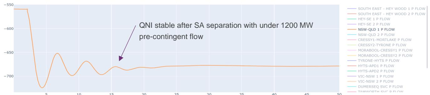
In the full OPDMS model, QNI appeared to enter an unstable condition almost immediately after exceeding its export limit of 1,200 MW, at 1,400 MW. In the simplified model, however, QNI reached a peak flow of 1,460 MW with no instability and reached a settled point of 1,350 MW. QNI appeared to remain stable for this condition regardless of tuning.
