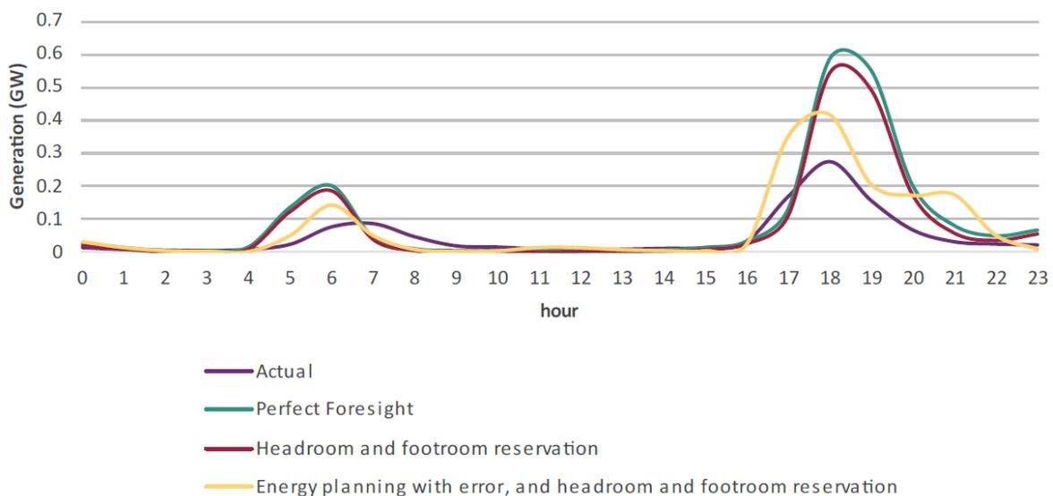
Adding in the ‘energy planning with error’ methodology makes the profile closer to actual output, but still overestimates the response of batteries to high price events. If AEMO relies on only these two methods (especially ‘headroom and footroom reservation’), the ISP model will provide an inaccurate picture of battery dispatch that overestimates the amount of battery
