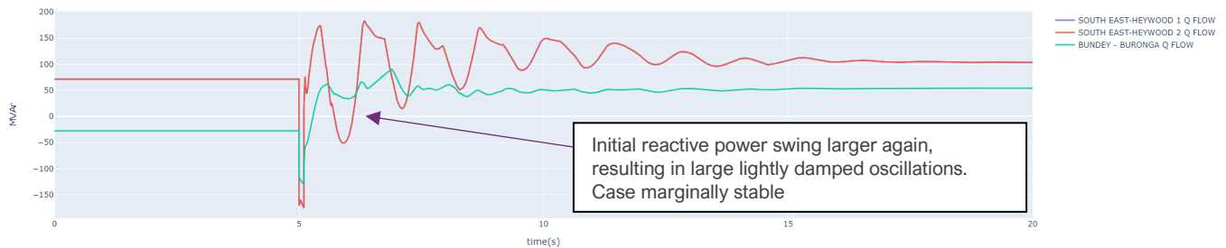
Figure 116 Case 5c8 interconnector reactive power response (MVAR)
