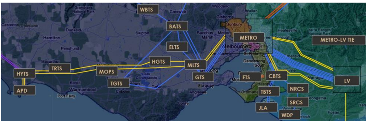
Figure 1 - 500 kV Transmission Backbone
