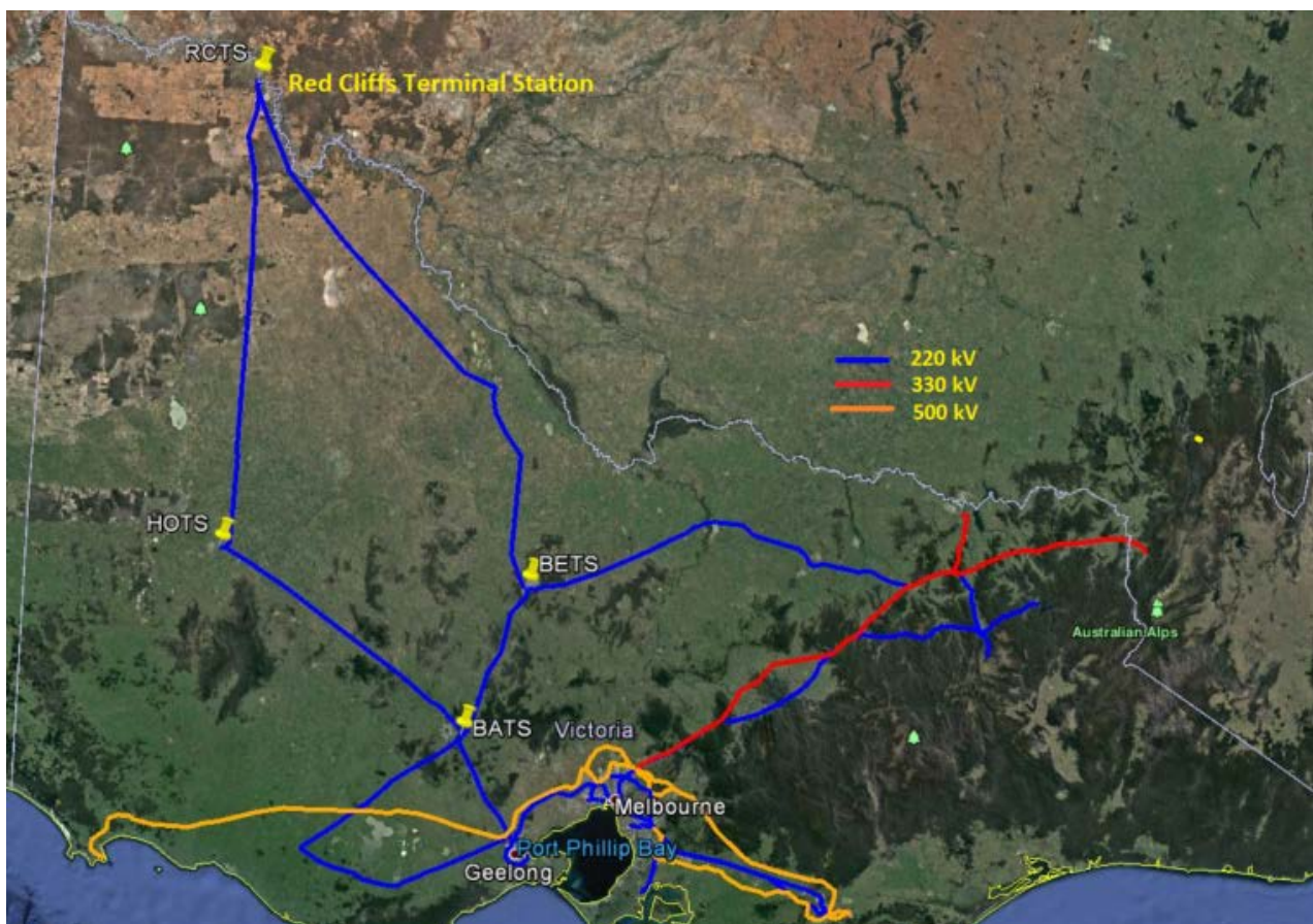
Figure 1 - Transmission network supplying RCTS
