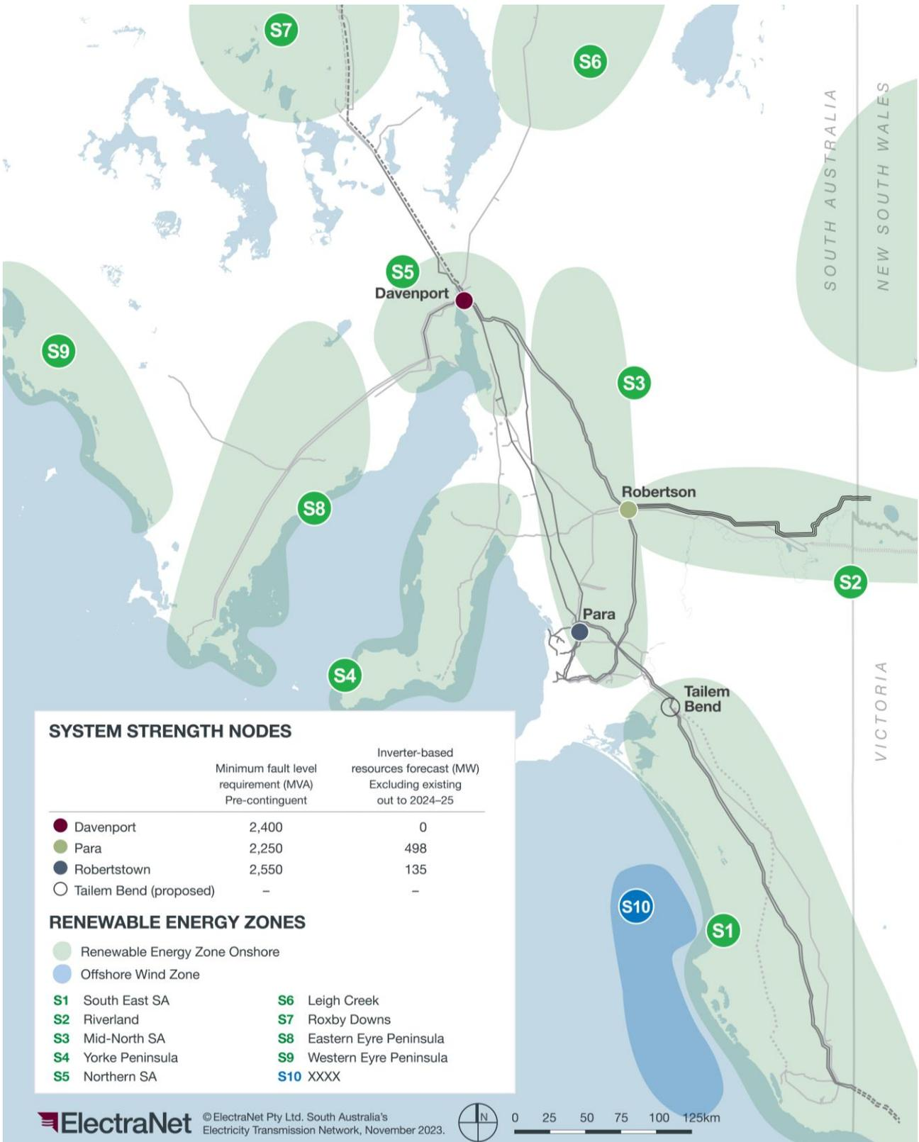
Figure 2: System strength node (SSN) locations and system strength standard in South Australia
