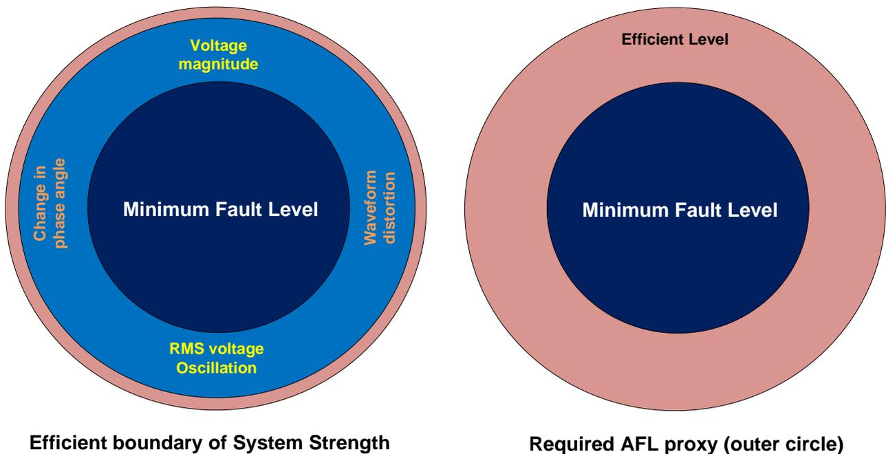
Figure 1: Conceptual representation for efficient level of system strength
