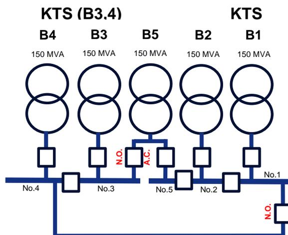
The summer cyclic rating of KTS (B1,2,5) with all plant in service is 509 MVA and with one of its three 220/66 kV 150 MVA transformers out of service, reduces to 339 MVA noting that the B5 transformer is also used as an auto-changeover spare to support the KTS (B3,4) group (as described above). Hence the available capacity across these two bus groups is intricately linked.
