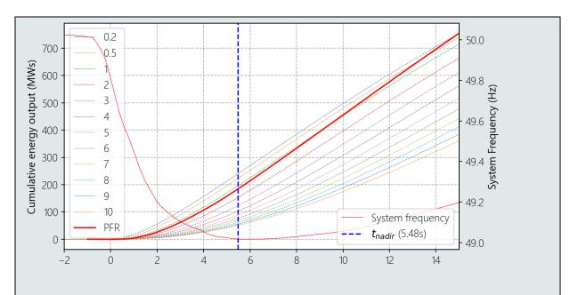
Figure E[4] Example of measured response against theoretical Response Profiles after integration.
