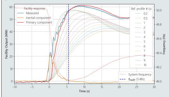
Figure E[3] Example of measured response against theoretical Response Profiles.
