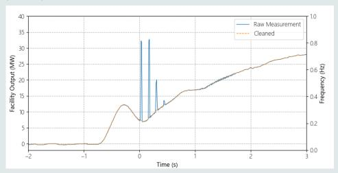
Figure E[2] Example of filtering erroneous data from a high-speed recording
