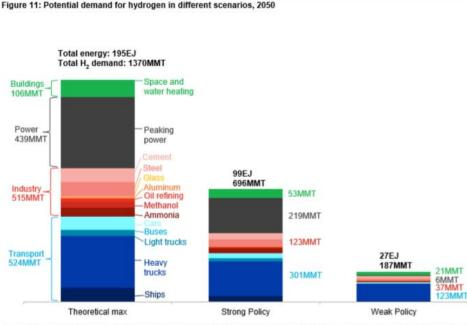
Source: BloombergNEF. Note: Aluminum demand is for alumina production and aluminum recycling only. Cement demand is for process heat only. Oil refining demand is for hydrogen use only. Road transport and heating demand that is unlikely to be met by electrification only: assumed to be 50% of space and water heating, 25% of light-duty vehicles, 50% of medium-duty trucks, 30% of buses and 75% of heavy-duty trucks.
